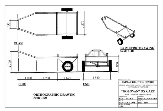
A complete set of plans and specifications for the construction of the Golovan ox cart and for a smaller version using two donkeys are available.
