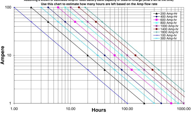
Assuming a known or estimated Amp-hr rated Battery Bank Capacity or State-of-Charge (what's left at the time)
