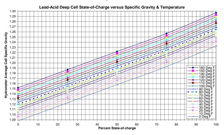
Lead-Acid closed Gel Cell State-Of-Charge measurements during discharge (Use 24hr rate as resting or no flow voltages)
