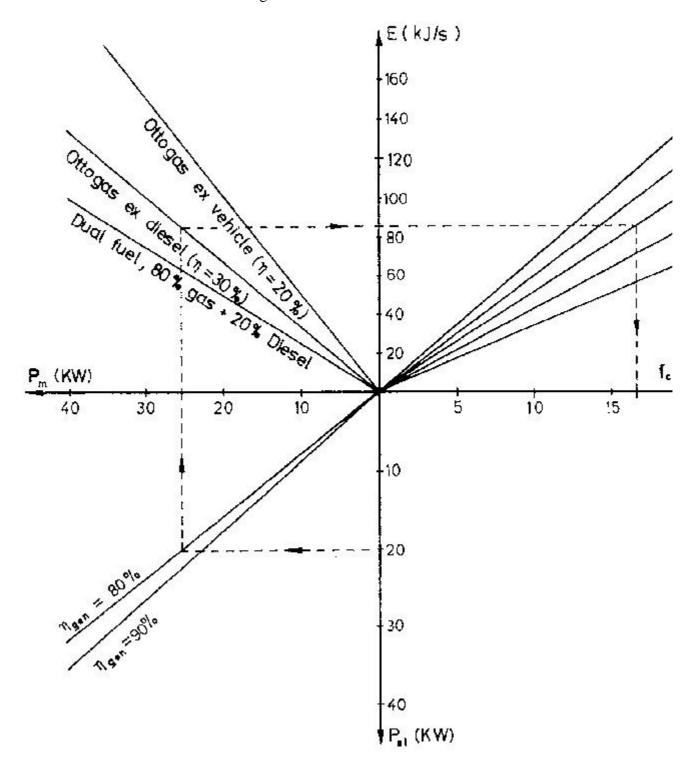
Fig. 7.9: Nomogram for the relation of fuel consumption/fuel demand fc, biogas quality  $\mathrm{CH_4\%}$ , fuel energy flow E, type of engine used, mechanical power output Pm, electric generator efficiency ngen, and electric power output Pel. Basic gas data assumed: temperature 25 °C, pressure 960 mbar, ref. humidity 100%.
