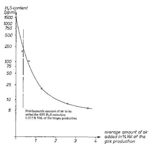
b) H<sub>2</sub>S reduction from initially 1500 ppm as a function of added air.
