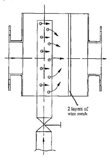
Fig. 5.5: Mixing chamber with gas distribution pipe and wire mesh for intensive mixing
