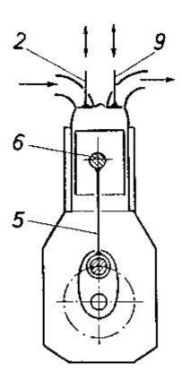
Fig.31:Principal scheme of a 4-stroke engine.1 piston, 2 inlet valve, 3 cylinder, 4 combustion chamber, 5 connection rod, 6 gudgeon pin, 7 crankshaft, 8 flywheel, Q head rejected (cooling).
