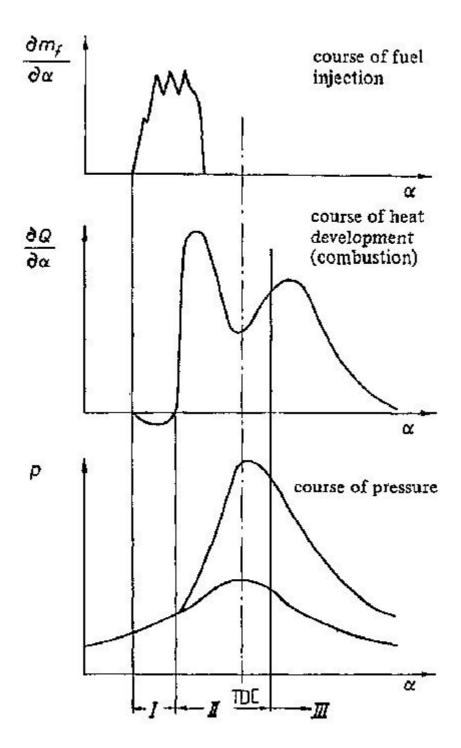
Fig. 3.9: Courses of fuel injection, combustion and pressure as a function of the crank angle a
