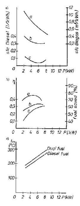
Fig. 5.12: Performance charts of a 10 kW single cylinder gas engine with biogas at n=1500 min<sup>-1</sup> (from[11]).
