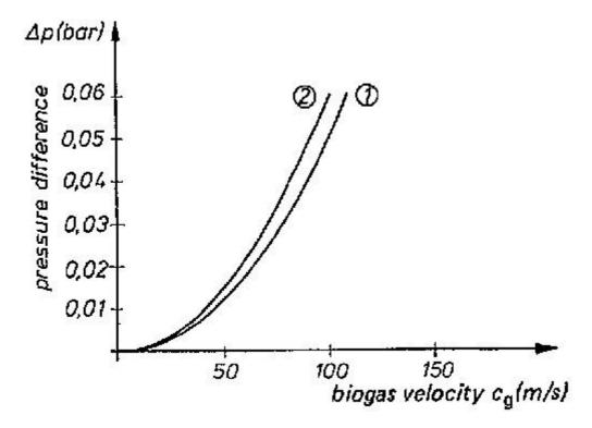
Fig. 6.4: Biogas flow through a nozzle cg as a function of the active pressure difference /p.
