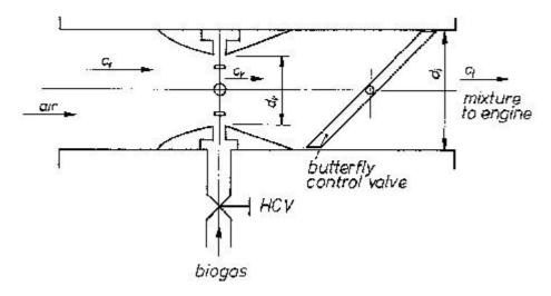
Fig. 6.2: Venturi mixer with gas supply through several bores.
