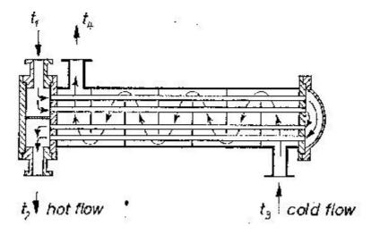
Fig. 8.2: Principial scheme of heat exchanger (mixed flow type)
