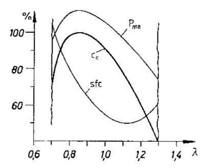
Fig. 3.4: Mean effective pressure Mme, combustion velocity  $c_c$  and specific fuel consumption sfc as a function of excess air ratio 1
