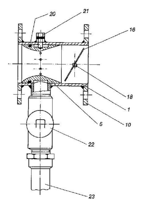
Fig. 3: Venturi mixer assembly
