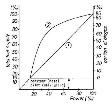
Fig. 5.9: Fuel supply vs. power output Diesel pilot fuel constant, biogas controlled (manualy or automaticaly) according to power demand.
