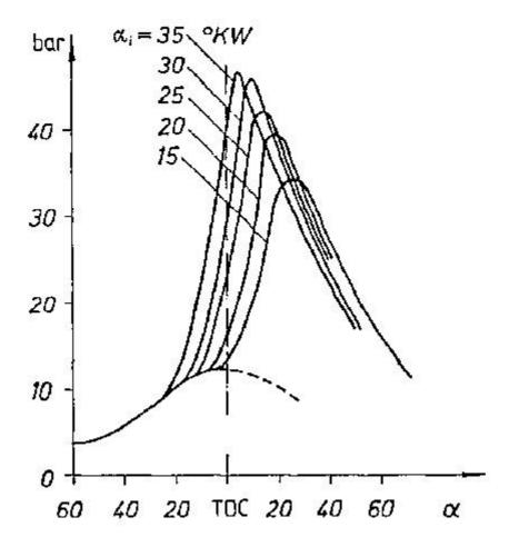
Fig. 3.5: Course of pressure as a function of the crank angle a (point) of ignition a;
