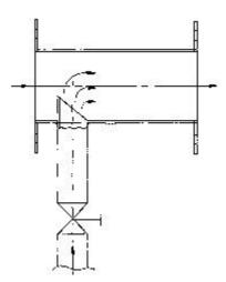
Fig. 5.4: T-joint mixer with oblique, protrunding gas inlet
