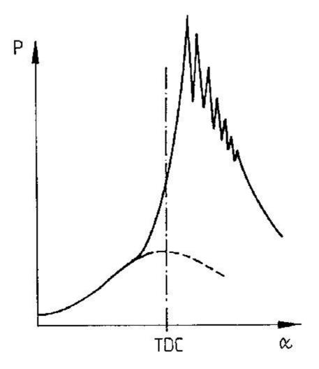
Fig.4.4: "Knocking" in a p, alfa-diagram of an engine
