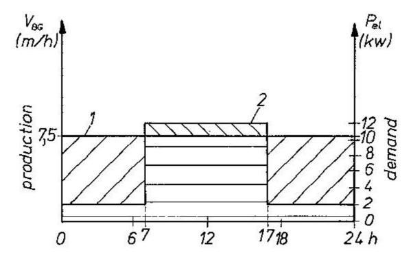
Fig. 7.14: Daily profiles: 1 biogas and potential power production, 2 electric power demand (refers to example)
