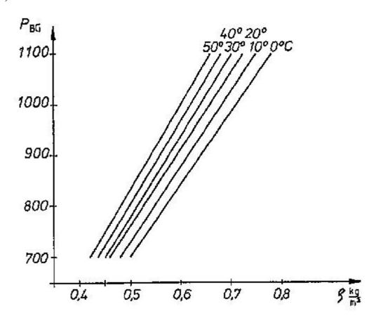
Fig. 4.1: Density r of CH<sub>4</sub> as a function of biogas pressure and temperature
