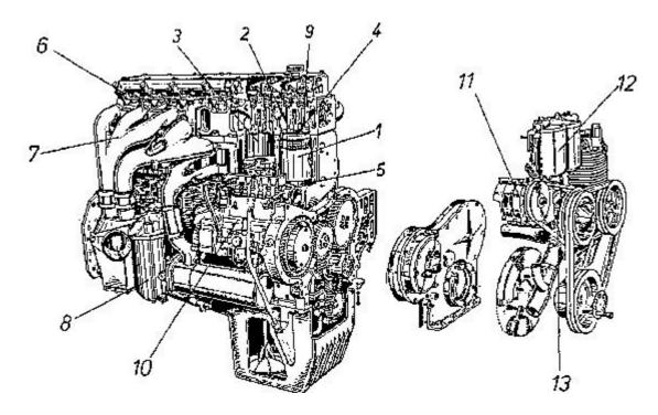
Fig. 3.7: 6-cylinder diesel engine, partly opened (MAN).
