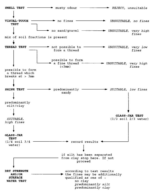
This field testing tree diagram illustrates one sequence in which the field tests may be carried out. This diagram does not include every possible field test but should illustrate that basic soil selection is possible if the tests are used coherently in a logical order.
