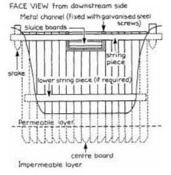
This design also makes a good weir on a narrow watercourse, as long as a breakwater is placed below the downstream face. More often it is provided with a sluice opening to control water levels, as shown in the diagram, in which case no other overflow is required.
