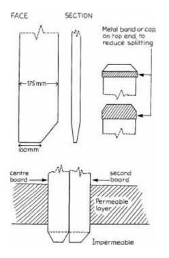
8. The dam must be properly keyed into the bank. This means driving the last board on each side down through the bank so that at least half its width is in the bank. Where the bank is too hard for this, make a water-tight corner instead, by driving in a couple of boards at right angles to the line of the dam where it meets each bank. Set the chamfer away from the dam so that the corner boards are driven tight against the last board in the dam itself.
