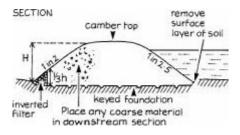
The diagram below shows a homogeneous dam on permeable soil, with a cut-off.
