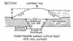
Homogeneous dams are constructed of impermeable soil throughout. This is the cheapest method if the soil is suitable, i.e. well graded with 20%-30% clay and with the non-clay fraction containing a fairly high proportion of coarser particles to increase stability and aid compaction. The clay content must not be too high or the soil will shrink on drying and be unstable.
