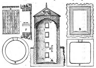
Fig. 168. Construction of circular, all-stone silo. (King.)
