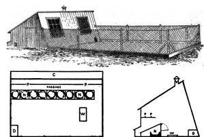
Fig. 201. House and yards for confined fowls: This house is so arranged as to be easily cleaned from the outside, the droppings falling into a trough at the rear, the floor under the roost being on an incline. C. incline; P.P., roosts; N.N., nests; D, dust box; W, water trough; V, ventilator.
