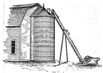
Fig. 169. Stave silo, 12 feet diameter, 24 feet high; capacity, 50 tons. (Elias.)
