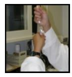
The hexane phase is easily removed by using a pippet.
