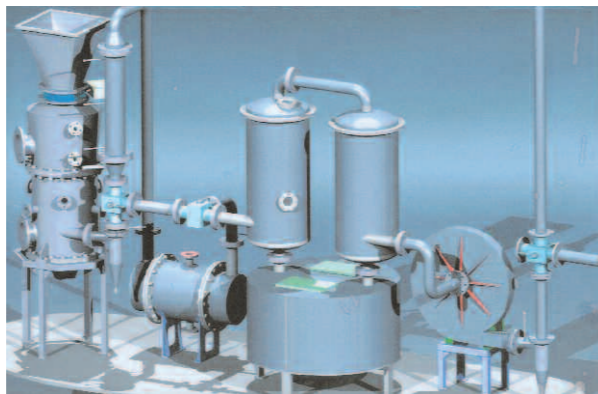
Figure 3: Pilot scale downdraft biomass gasifier
