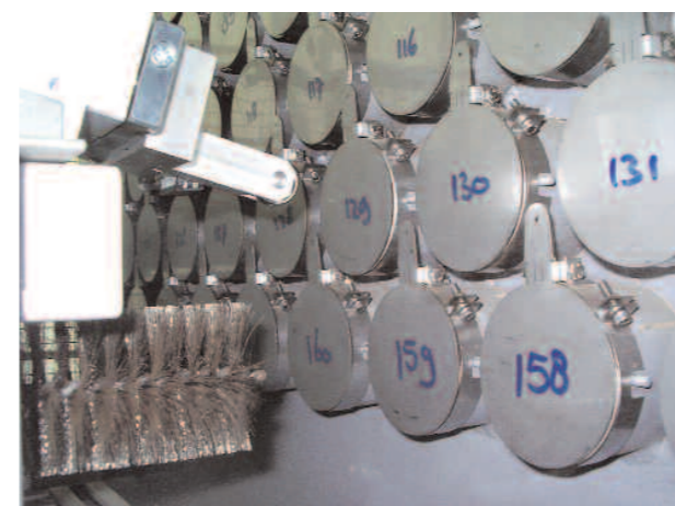
Figure 5: Lance with brush in front of opener/shutter.
