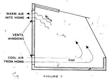
house for heating. Without any mechanical devices this natural cycle will function continuously on any relatively sunny day (see this figure as well as figure 5 on page 10). Two additional benefits are provided by this type of air circulation. The plants in the unit convert carbon dioxide into oxygen-rich air for the home, a definite health benefit for the occupants. Also, in areas of the country with very low humidity, the added moisture from the greenhouse
