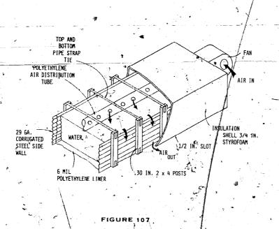
terials and assorted configurations of black poly absorbers, mesh shadecloth and clear poly coverings are examined. Flow rates and efficiencies of heating and losses are determined. In the system, the warm water is then drained off the bottom of the collector and stored in an insulated tank that fits under the greenhouse benches. The warm water in the tank heats air moving through a poly tube which in turn heats the greenhouse. See Figure 107
