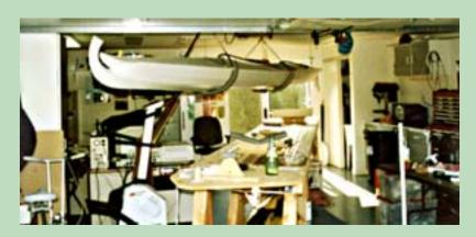
The most critical part of this operation is to have the frame supports cut out and precisely placed on the strong-back (work bench)
