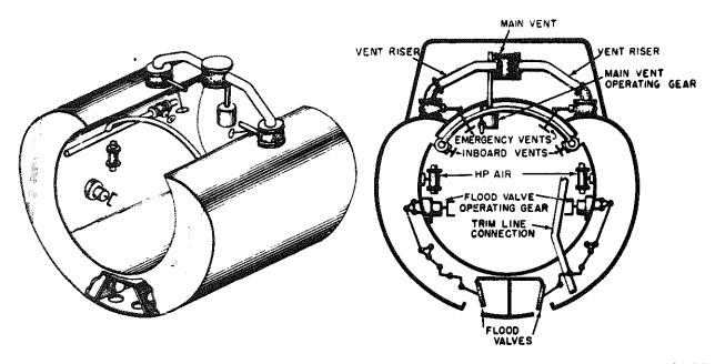
Figure 10-13.—Submarine special ballast tank (safety tank).
