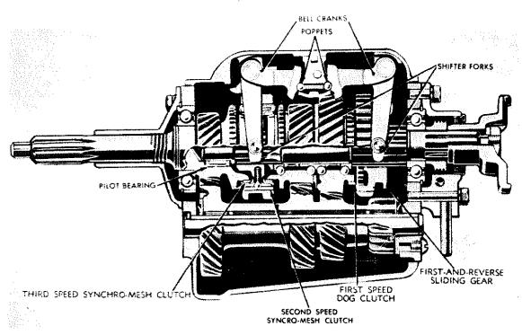
Figure 14-10.—Synchromesh transmission arranged for steering column control.
