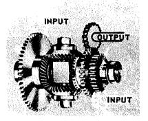
Figure 11-13.—Any of these three hookups can be used.
