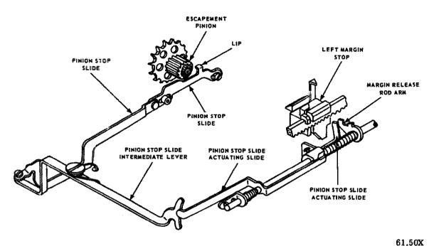
Figure 12-16.-Pinion stop slide mechanism.
