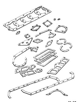
81.52 Figure 13-12.—Engine overhaul gasket kit.
