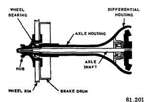
Figure 14-22.—Three-quarter floating rear axle.
