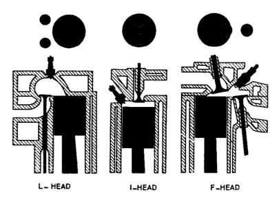
Figure 13-8.-L-, I-, and F-valve arrangement.
