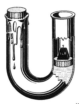
Figure 10-7.—The liquid transmits the force.
