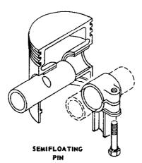
Figure 13-17.—Piston pin types.
