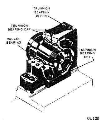
Figure 11-6.—Radial-thrust roller bearing.
