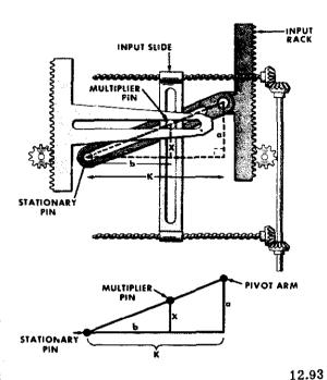
Figure 15-6.—Screw type multiplier—
