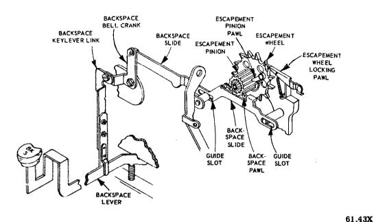
Figure 12-9.-Back spacer mechanism.
