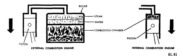
Figure 13-1.-Simple external and internal combustion engine.
