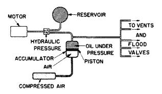
Figure 10-14.—This keeps pressure on tap.
