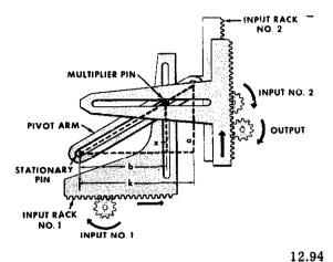
Figure 15-7,-Rack type multiplier.
