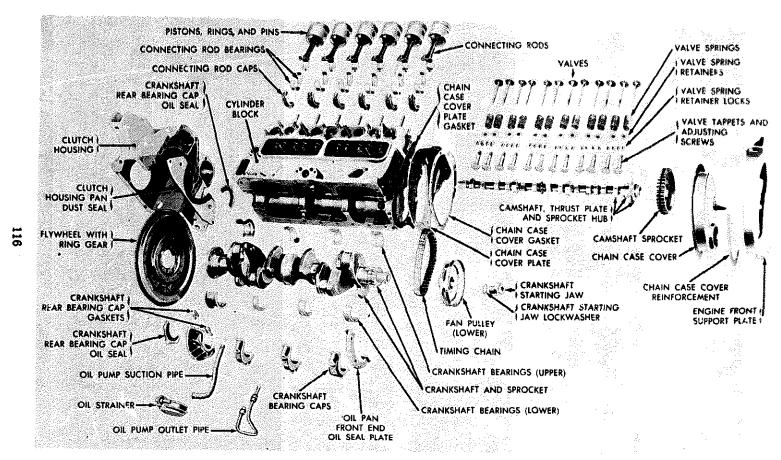
Figure 13-9.—Cylinder block and components.
