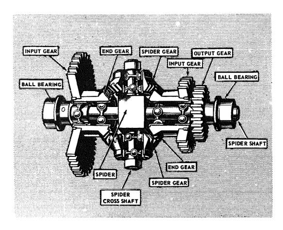
Figure 11-8. - Bevel gear differential.
