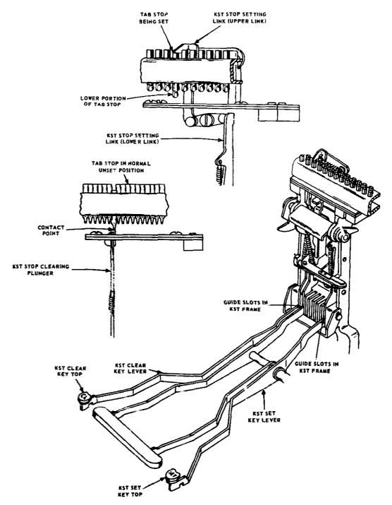
Figure 12-11.—Tabulator stop setting mechanism.
