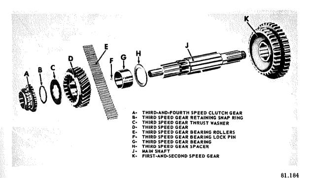
Figure 14-8.-Disassembled main shaft assembly.
