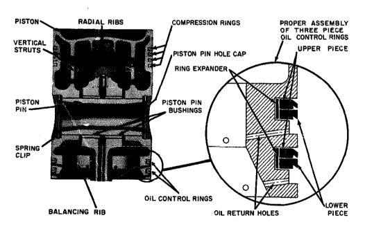
Figure 13-15.—Piston assembly of General Motors series 71 engine.
