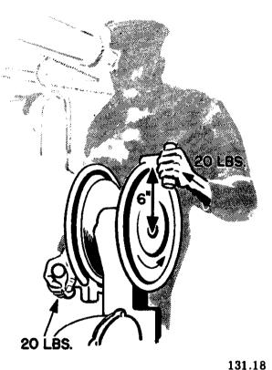
Figure 3-10.—Developing a torque.
