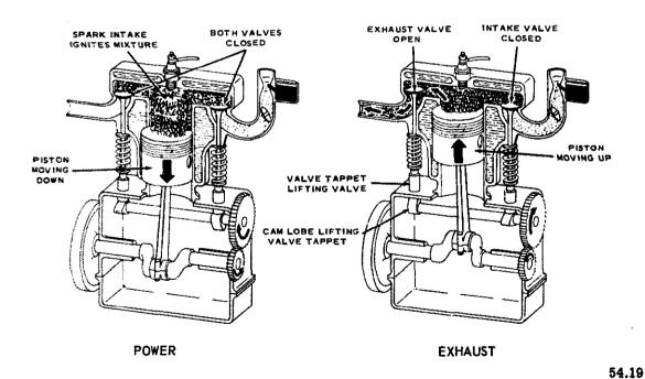
Figure 13-4.—Four-stroke cycle in a gasoline engine.
