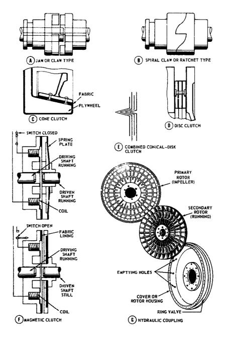
Figure 11-25. - Types of clutches.
