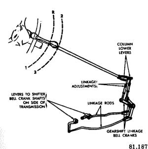
Figure 14-11.—Steering column transmission control lever and linkage.
