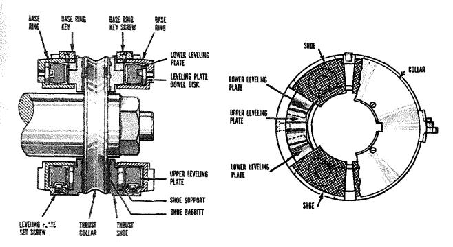
Figure 11-2.-Kingsburg pivoted-shoe thrust bearing.
