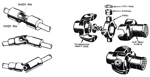
Figure 11-17.—Universal joint (Hooke type). Figure 11-18.—Ring and trunnion universal joint.
