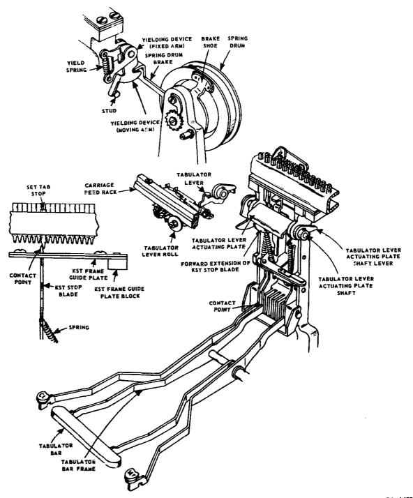
Figure 12-10.—Tabulator mechanism.
