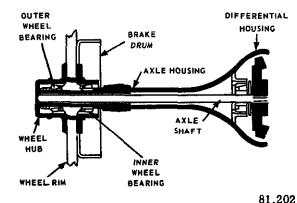
Figure 14-23.—Full floating rear axle.
