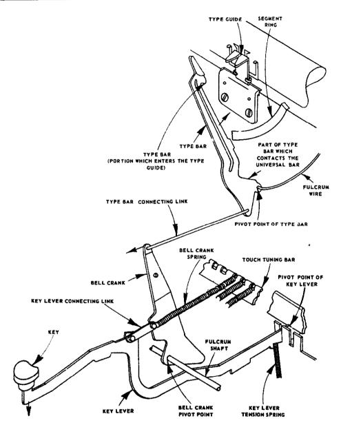
Figure 12-6.—Type bar action mechanism.
