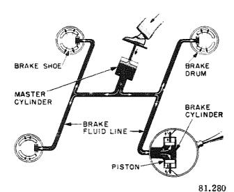
Figure 10-6.-Hydraulic brakes.
