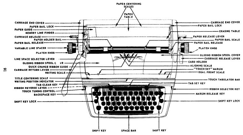
Figure 12-4.—External parts of a standard typewriter.
