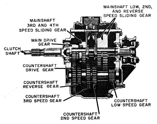
Figure 14-5.-Four-speed truck transmission.
