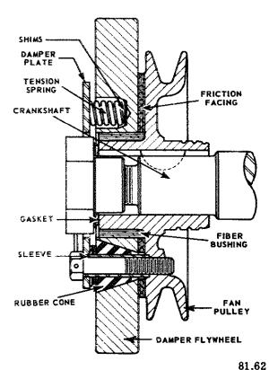
Figure 13-21.—Sectional view of a typical vibration damper.
