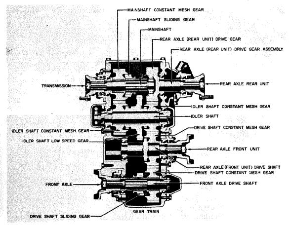
Figure 14-14.—Cross section of a 2-speed transfer case.
