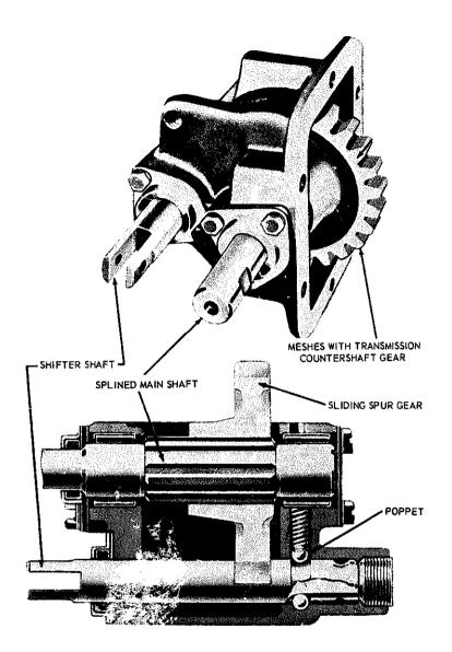
Figure 14-15.-Single speed, single gear, power takeoff.
