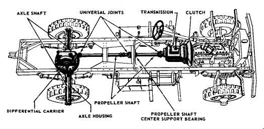
Figure 14-1.-Type of power transmission.
