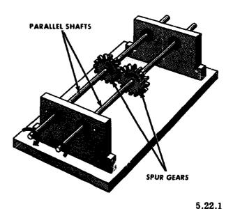
Figure 6-2.—Spur gears coupling two parallel shafts.
