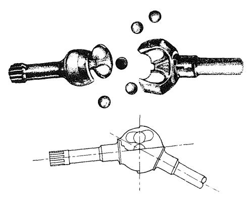
Figure 11-19.-- Bendix-Weiss universal joint.
