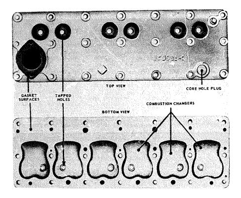
Figure 13-10.--Cylinder head for L-head engine.
