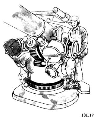
Figure 3-9.—A pointer's handwheel.
