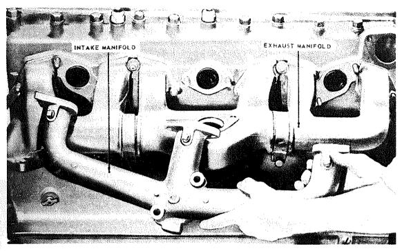
Figure 13-11.—Intake and exhaust manifolds.
