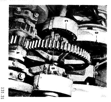
Figure 6-14.-An anchor winch
