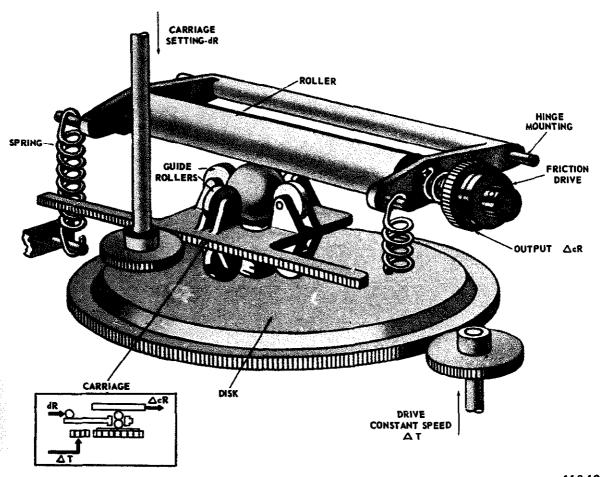
Figure 15-15.—The disc type integrator.
