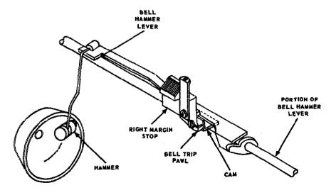
Figure 12-13.-Bell ringer mechanism.
