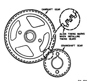
81.69 Figure 13-27.—Timing gears and their markings.
