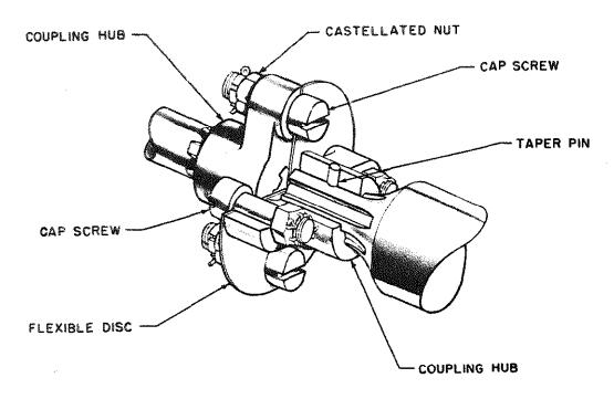
Figure 11-21.—Flexible coupling.
