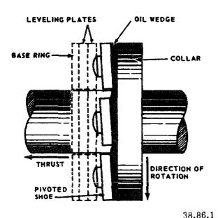
Figure 11-3.—Diagrammatic arrangement of a Kingsburg thrust bearing, showing oil film.
