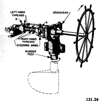
Figure 5-8.—The screw gives a tremendous mechanical advantage.
