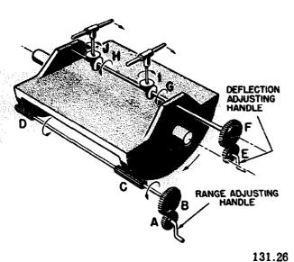
Figure 6-8.—Gears change direction of applied motion.
