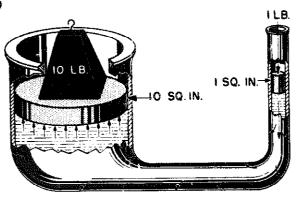
Figure 10-9.-A mechanical advantage of 10.
