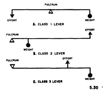
Figure 1-2.—Three classes of levers.
