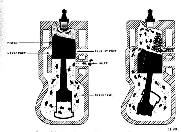
Figure 13-5.—Events in a two-cycle, internal combustion engine.
