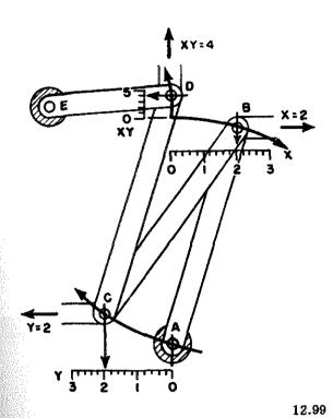
Figure 15-12.—Multiplying linkage.
