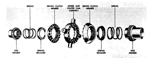
Figure 14-20.-No spin differential-exploded view.
