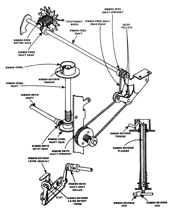
Figure 12-7.-Ribbon feed mechanism.
