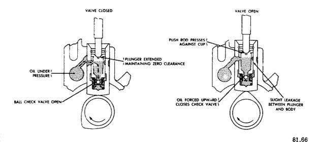
Figure 13-26.—Operation of a hydraulic valve lifter.
