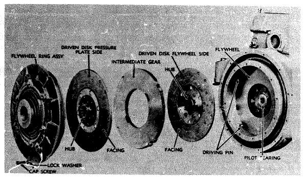
Figure 14-4.—Double disk clutch—exploded view.
