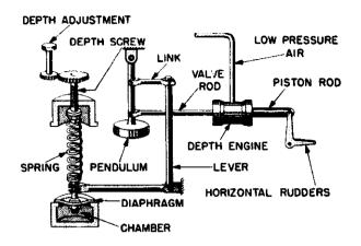
Figure 10-3.-Inside a torpedo.
