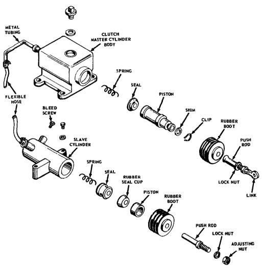
Figure 14-3.—Master cylinder, slave cylinder and connections for standard hydraulic clutch.
