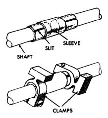
Figure 11-15.—Sleeve coupling.
