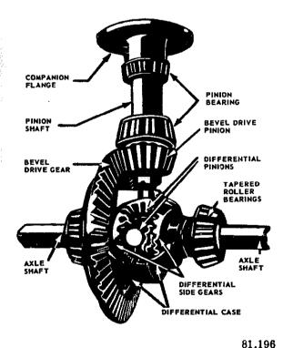
Figure 14-18.—Differential with part of case cut away.
