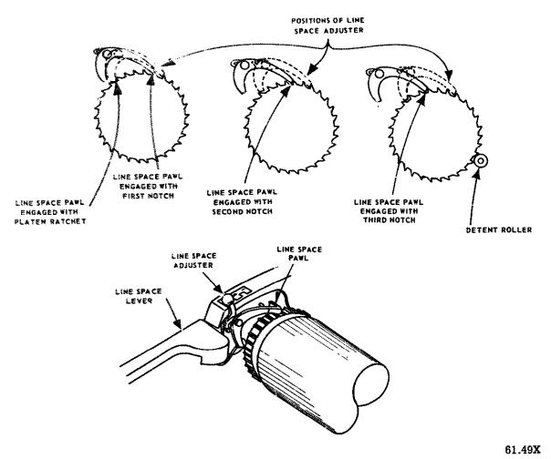
Figure 12-15.—Line space mechanism.
