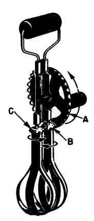
131.25 Figure 6-1.—A simple gear arrangement.
