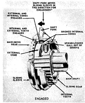
Figure 14-9.-Synchromesh clutch-disengaged and engaged.
