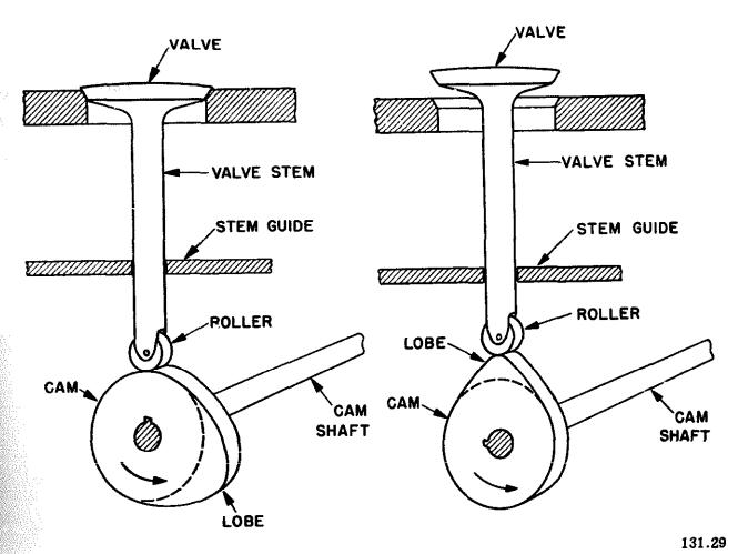
Figure 6-12.—Cam-driven valve.
