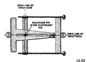
Figure 15-5.—Screw type multiplier—zero position.
