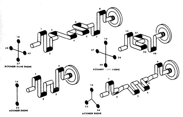
Figure 13-20.-Crankshaft and throw arrangements commonly used.
