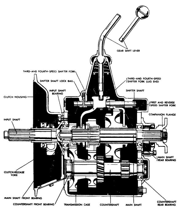
Figure 14-7.—Constant-mesh transmission assembly—sectional view.
