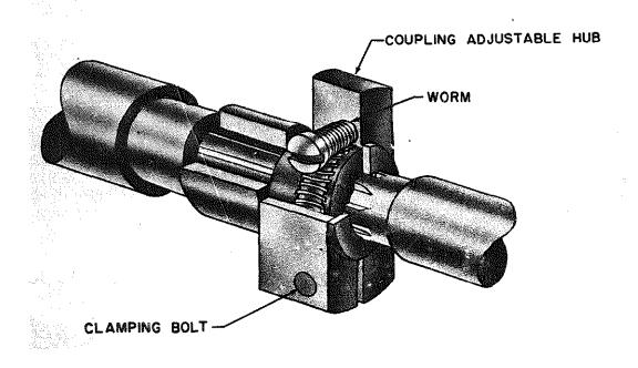
Figure 11-22.—Adjustable (vernier) coupling.
