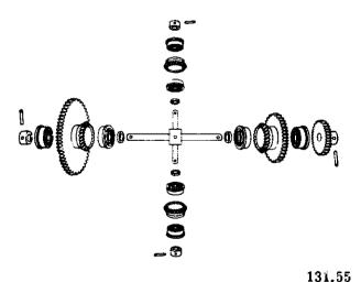
Figure 11-9.—Exploded view of differential gear system.
