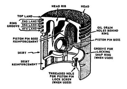
Figure 13-14.—The parts of a piston.
