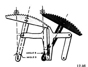
Figure 15-9.—Multiplying with the sector type multiplier.
