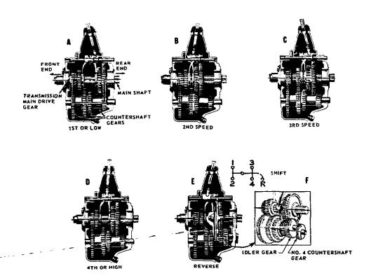
Figure 14-6.-Power flow through a 4-speed transmission.
