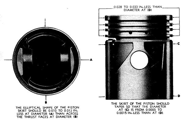
Figure 13-16.—Cam-ground piston.
