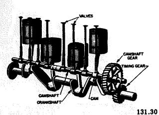
Figure 6-13.—Automobile valve gear.
