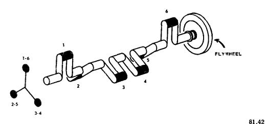
Figure 13-6.-Crankshaft for a six-cylinder engine.
