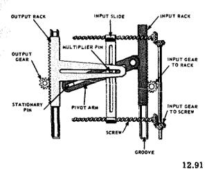
Figure 15-4.—Screw type multiplier.
