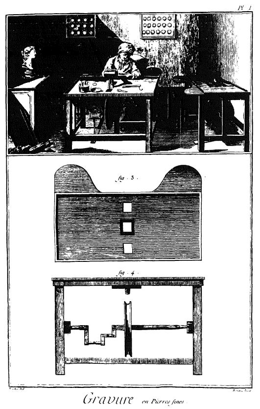
Figure 1-15 A machine for engraving fine stone (Compliments of Lehigh University, Honeyman Collection)
