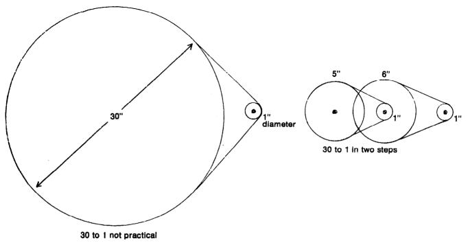
Figure 4-5 Pulley system
