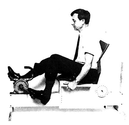
Figure 2-10 Rotary hand pump connected to pedal operation, mounted on fully adjustable sliding-seat (Courtesy of Autometruc Pumps, Ltd.)
