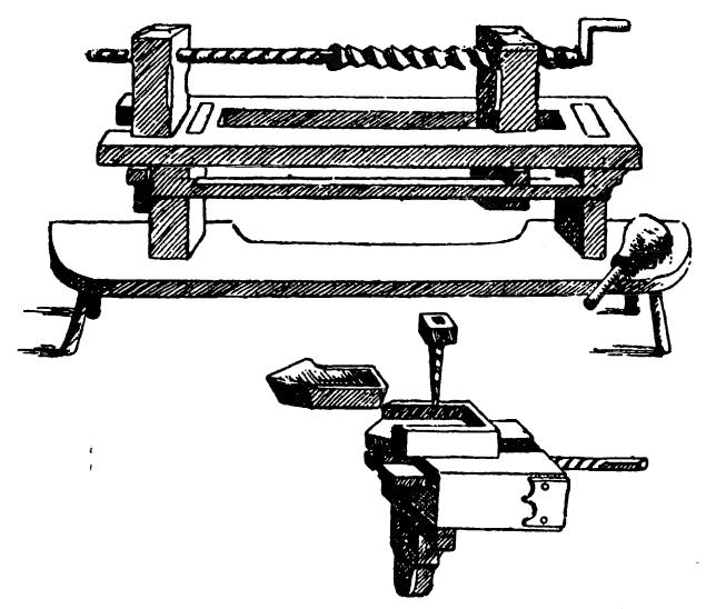
Figure 1-6 Screw-cutting lathe (Courtesy of Friedrich Klemm)
