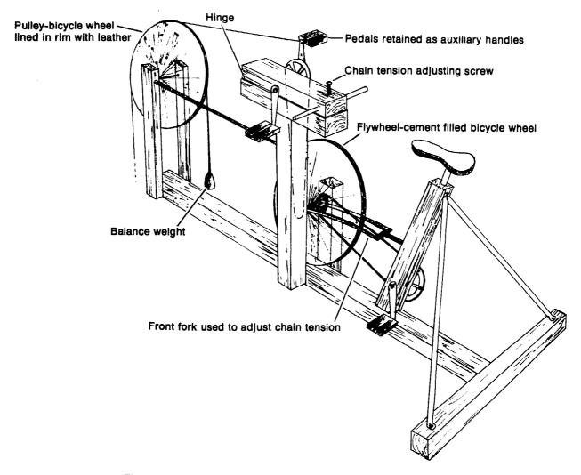
Figure 2-23 Pedal drive for low-lift borehole pump (prototype)
