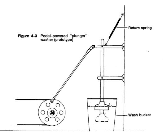
The parallelogram linkage keeps the plunger aligned with the bucket. This system works well. Five minutes of leisurely pedaling will wash 5 lbs. of clothing. Drain the tub and refill with water. Pedal for two or three minutes more and drain. The clothing will have to be rung out either by hand or by using a roller-type wringer. Sears carries a suitable wringer in the big catalog (11K 577OC).
