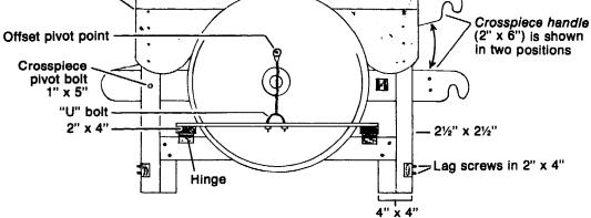
Figure 5-10 Side view of band saw
