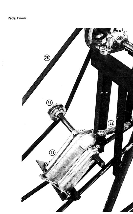
**Figure 3-31** Research and Development personnel adapted a one-piece grinder shaft assembly to perform the task of an idler—a mechanism to remove slack from the V-belt.
