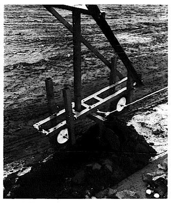
Figure 3-23 Frame with plow attachment
