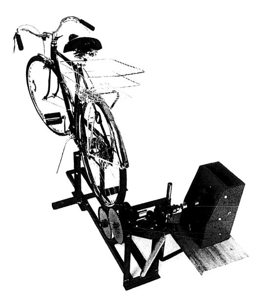
**Figure 3-36** Bicycle rests on the two frame mounts and is secured in place with two turnbuckles. A converted electric grain mill sits on the adjustable table and its drive shaft is clamped inside the chuck.
