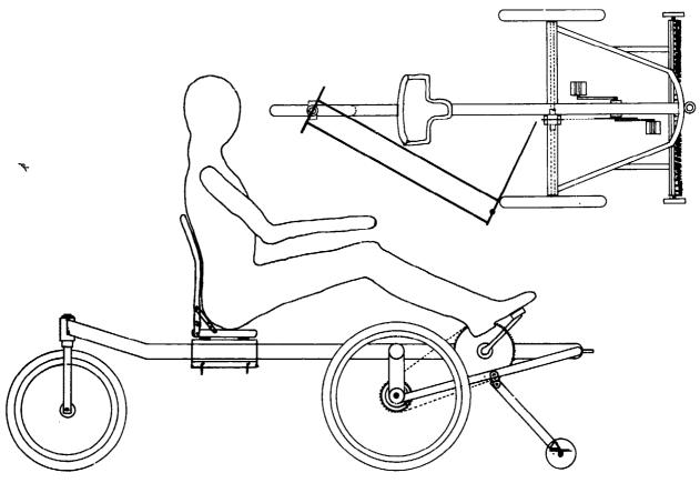
Figure 6-3 Preliminary drawing for pedal-powered lawn mower
