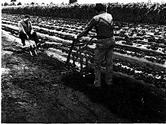
Figure 3-21 The winch is a two-man operation. pedaler. Welded on the handle is a metal extension which wedges against the tooth of a sprocket (one side of the spool) from the force of a spring to brake the spool. The winch assembly is built into a frame which also supports the seat.
