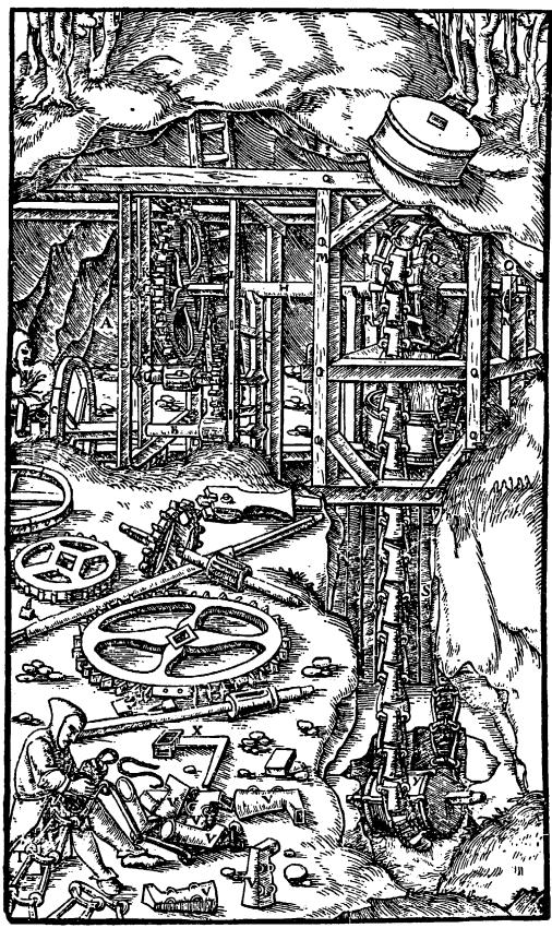
Figure 1-3 Bucket-chain water lifter (Courtesy of Friedrich Klemm)
