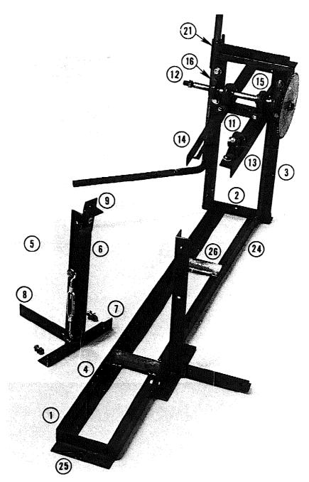
Figure 3-33 The rear-wheel adapter model consists of three components: floor frame and rear uprights, bicycle frame mounts, and spring-loaded power arm.
