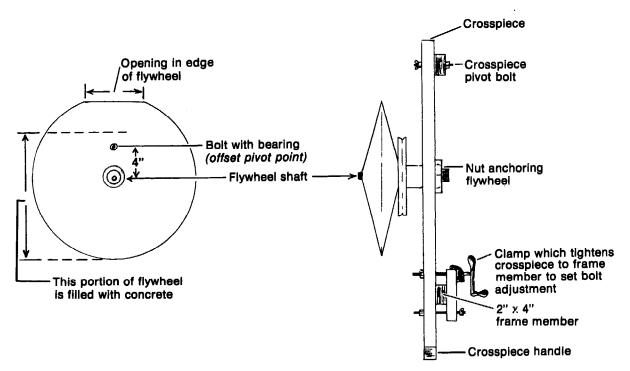
Figure 5-11 Left—flywheel; right—top view of flywheel and crosspiece
