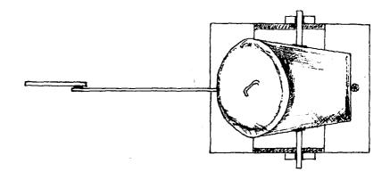
Figure 4-4 Trash can washing machine
