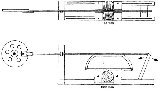
Figure 4-6 Pedal-driven wood saw (prototype)
