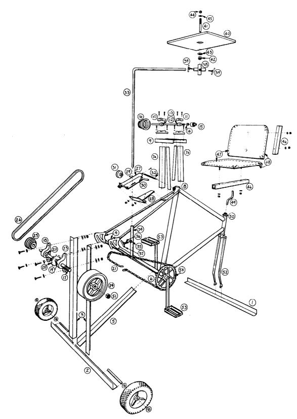
Figure 3-25 Exploded view of homemade Energy Cycle
