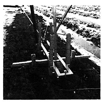
**Figure 3-24** The winch performs gardening tasks on 12-inch centers rather than 24-inch, thereby increasing the productivity of the garden.
