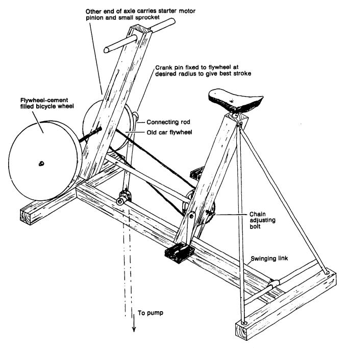
Figure 2-24 Pedal drive for deep borehole pump (prototype)
