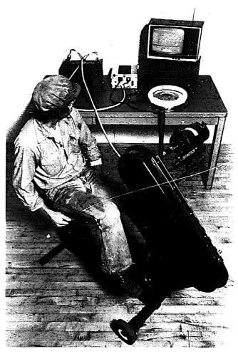
Figure 3-14 Generating electricity with the Energy Cycle
