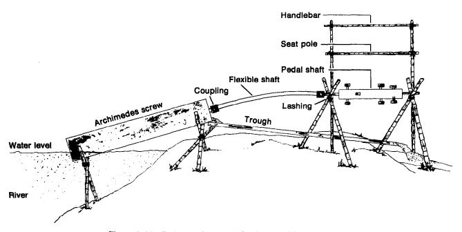
Figure 2-21 Prototype for a pedal-driven Archimedes screw
