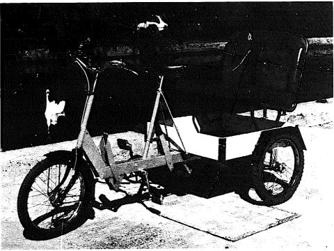
Figure 2-8 Oxtrike with temporary seat
