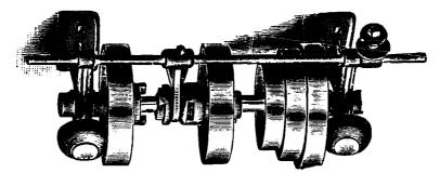
The above cut represents a countershaft for No. 4 and  $4\frac{1}{2}$  lathes. The pulleys on countershaft are  $7x1\frac{1}{2}$  inches, and should be speeded 250 revolutions.
