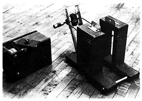
Figure 3-37 The Thompsom Mill, manufactured in Mesa, Arizona, can be operated electrically or by pedal. The power takeoff frame is limited in that it will support only a single- or three-speed bicycle.
