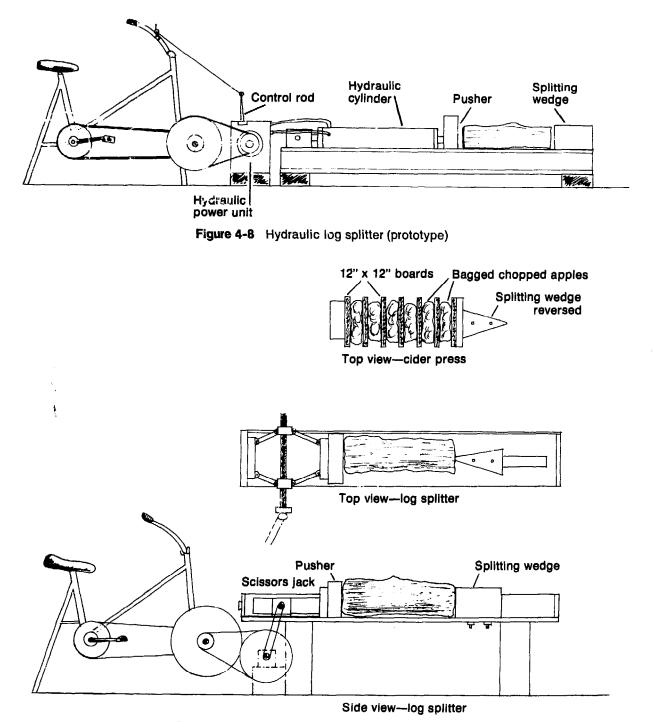
Figure 4-9 Scissors jack log splitter and cider press
