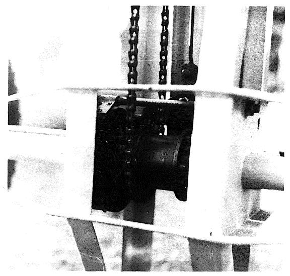
Figure 2-6 Back axle drive of Oxtrike
