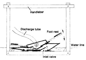
Figure 2-17 Schematic drawing of a bellows pump
