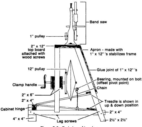
Figure 5-9 End view of band saw
