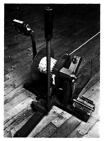
Figure 3-20 Close-up of brake handle and metal extension that wedges against the teeth of the sprocket to brake the spool
