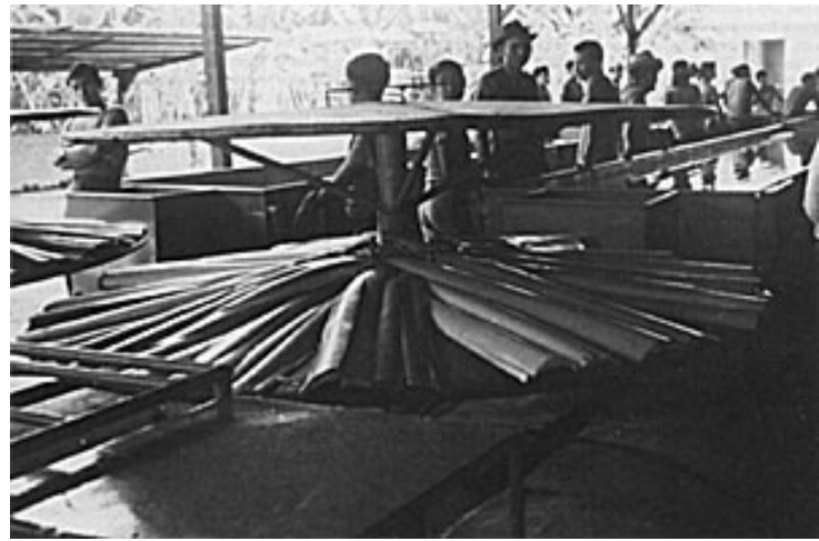
Fig. 12 Banana pseudostem pad on inspection-turntable, Hacienda Secadal, Ecuador.
