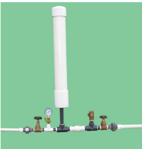
Figure 1. A 3/4-inch homemade hydraulic ram pump made with PVC fittings. Water flows from right to left during operation. Photo credit: W. Bryan Smith, Clemson University.
