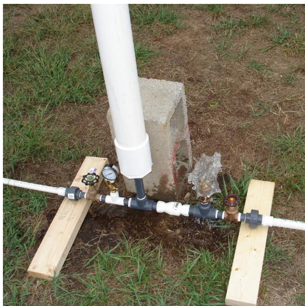
Figure 14. A 3/4-inch hydraulic ram pump (Design 1) in operation. The image was taken just at waste valve closure. The concrete block is in place to support the air chamber. Photo credit: W. Bryan Smith, Clemson University.
