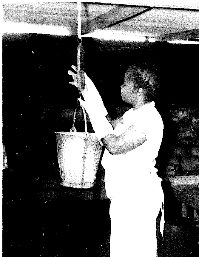
Plate 12: Weighing caustic soda with a spring balance
