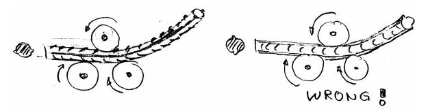
Figure 4: Proper feeding of the reinforcement bars into the circle mashine
