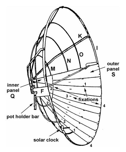
Figure 13: The fixation points of the aluminium panels
