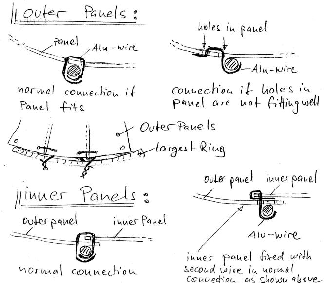
Figure 9: Some tricks, whoh to fix the panels with the wire if the holes in the panels do not fit perfectly
