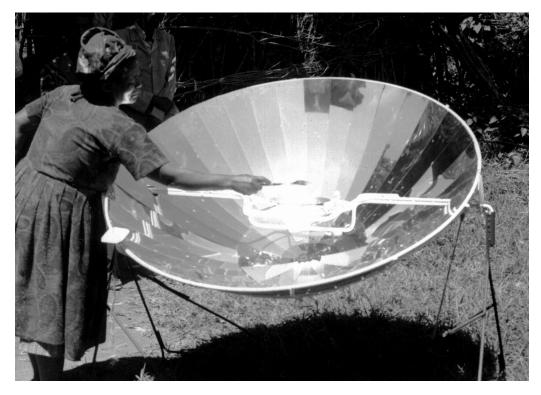
Figure 1: Roasting coffe with the AMSI solar cooker
