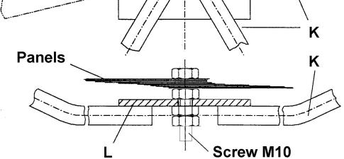
Figure 15: Fixation of the inner panels with an M 10 screw
