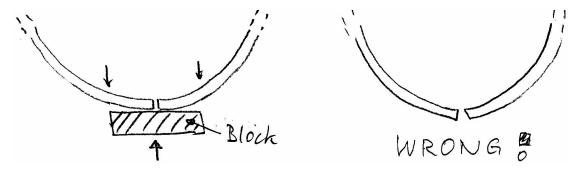
Figure 5: The closure of the rings by welding
