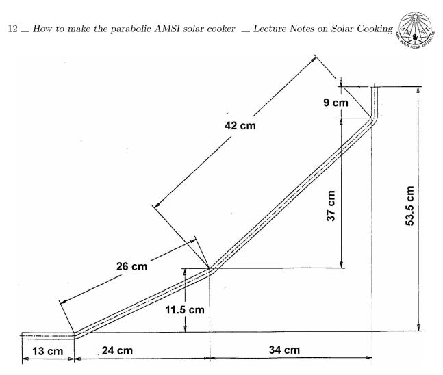
Figure 6: The measurements of the connection bar K
