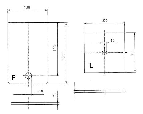
Figure 8: The sheet metal parts F and L
