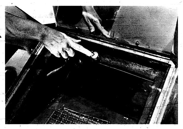
The finger is pointing to the shadow on the knob. Adjust the oven until the shadow disappears, the solar oven will then be pointing directly at the sun.
