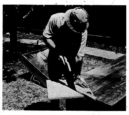
Dan using the clamped board guide to help saw the sides accurately.
