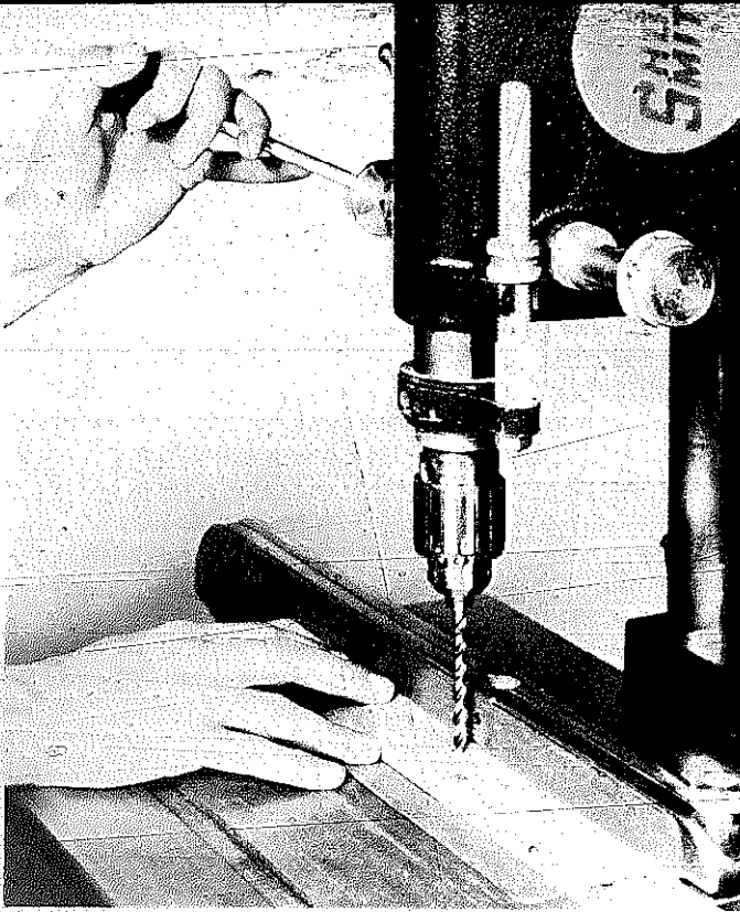
A fence, which doesn't have to be more than a straight piece of wood clamped to the table, is an excellent guide for maintaining hole edge-distance.
