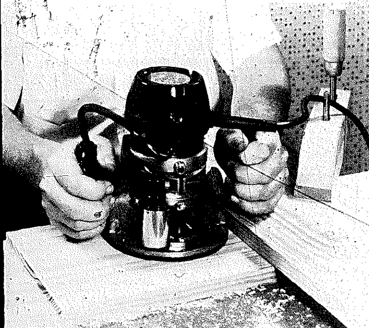
As in all woodworking, crossgrain cuts are the most difficult to do, especially when the wood has very prominent grain. Keep feed slow and depth of cut reasonable.
