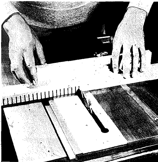
A miter-gauge extension jig is nice to have so you can position work for automatic, equal spacing of the kerfs. A multiple-blade setup would speed such operations.
