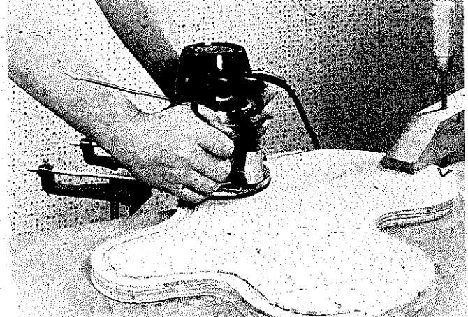
The router works well on plywood, but on deep cuts it's best to do the first cut just deep enough to get through the surface veneer. This approach will help appearance of the finished job.
