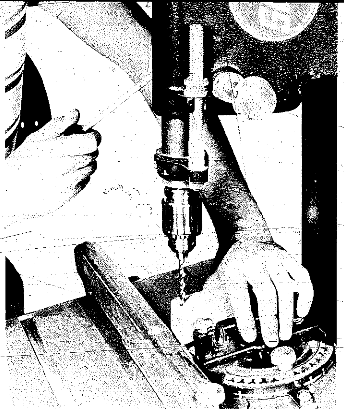
When rip fence and miter gauge are part of the table, they can be used to form jigs. Lacking such accessories, you substitute wood pieces to accomplish similar chores.
