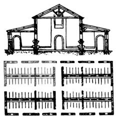
Fig. 98.—Ground-plan and Section of Industrial Stable, showing two double rows of horses between opposite sources of air supply. This is an aggravated condition of the bad arrangement shown in Fig. 94.
