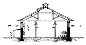
Fig. 23.—Transverse section of stable. Two horses are placed between opposite windows, heads to outer walls. The arrows indicate the direction of the wind.
