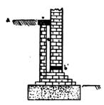
Fig. 82.—A Damp-proof Course. a. Ground level; b, vitrified work.
