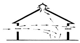
Fig. 7.—Direction taken by air currents with windward and leeward windows open.
