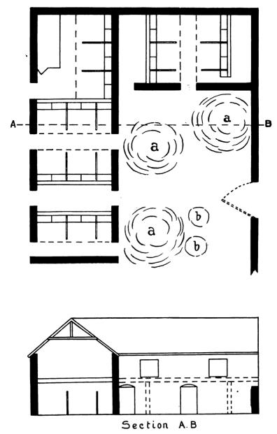
Fig. 135.—Ground-plan and Section of an Insanitary and badly-arranged Cow-house. It is overcrowded; lighting and ventilation are absent; the roof is low, as may be seen from the section A B, while in the yard the manure a, a, a is deposited anywhere (Lloyd).
