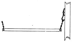
Fig. 121. - Army bail made of iron.
