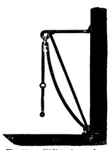
Fig. 114.—Sliding ring on bar (St. Pancras).
