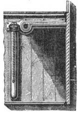
Fig. 115.—Noiseless fastening (Musgrave) for placing either under the manger or against the side of the stall, depending upon whether a single or double fastening is adopted.
