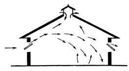
Fig. 9.—Direction taken by air currents when opposite windows are half open.
