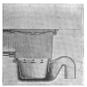
Fig. 164.—Fixed Syphon Stable Trap with removable bucket.
