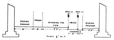
Fig. 131.—Arrangement of Cow-shed Floor as recommended by Lloyd.
