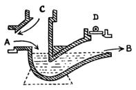
Fig. 157.—Buchan's Disconnecting Syphon. The sewage enters at A and escapes into the sewer pipe at B. D is an access opening in case of an obstruction. C communicates with the outside air, and ensures the air in the stable pipe being pure.
