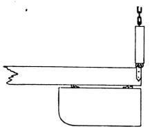
Fig. 124.—A compound bail with kicking-piece attached.
