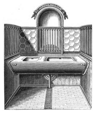
Fig. 112.—Manger fittings, with hay-rack let into the wall and manger sloping away from the knees (Musgrave).
