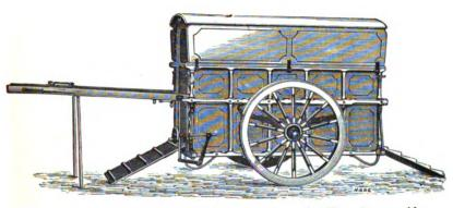
Fig. 215.—Ambulance for Animals for transit by road. There is a movable cover in this design, also a regulating screw lever for keeping the body of the cart level when travelling up or down hill (East Yorkshire and Crosskill's Cart and Waggon Co., Beverley).
