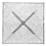
Fig. 153.-Loose Box Paving.
