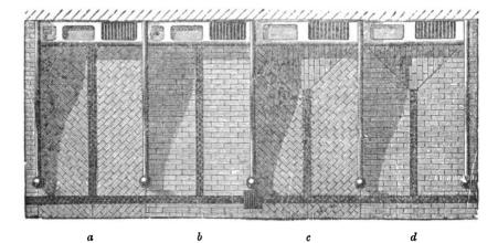
Fig. 152.—Methods of laying Paving Bricks in Stalls; b and d are good arrangements.
