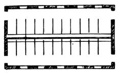
Fig. 94.—Ground Plan of Stable with double row, the horses' heads being turned towards the centre, which is a bad arrangement.
