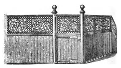
Fig. 106.—Loose Box Division, agreeing in design with Fig. 105.
