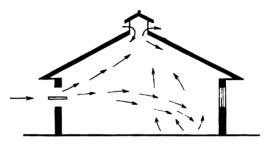
Fig. 6.—Direction taken by air currents with the windows open to windward.
