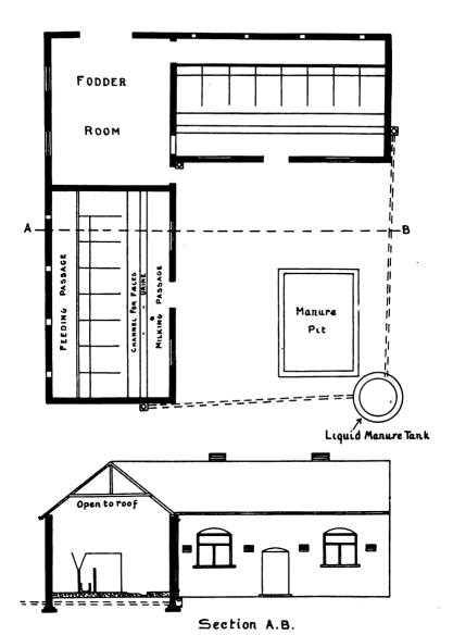
Fig. 136.—The same Cow-house shown in Fig. 135, but now remodelled so that it is converted into a sanitary and convenient building. Accommodation is only provided for half the number of animals, the building is
