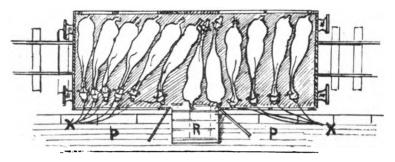
Fig. 214.—Diagram of truck loaded with horses. PP is the platform; R, the lamp leading into the truck. At XX stands a man to receive the head-ropes as the horses are loaded.
