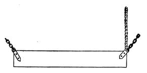
Fig. 123.—Simple plank bail, either suspended from above or from a heel post.
