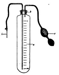
Fig. 66.—Apparatus for the injection of considerable quantities of toxin into the horse: a, Graduated cylinder closed by a rubber cork, b. Air is pumped into the constant pressure bulb e, and from this passes into the cylinder. The toxin is forced out through the needle at i (Levaditi).
