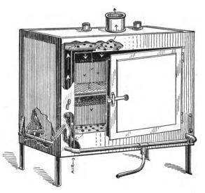
Fig. 48.—Oven for sterilization by hot air (Jordan).
