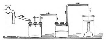
Fig. 51.—Apparatus for sterilization by filtration (McFarland).
