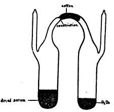
Fig. 69.—A tube used for the preservation of antitoxin by the Hygienic Laboratory of the Public Health and Marine Hospital Service: a, Serum scales, or antitoxin; b, phosphorus pentoxid, an active dehydrating agent (M. J. Rosenau, Bulletin No. 21, Hygienic Laboratory).
