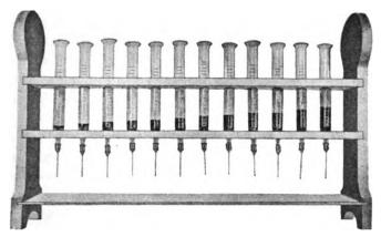
Fig. 70.—Battery of syringe tubes for testing the potency of toxin and antitoxin (Madsen).
