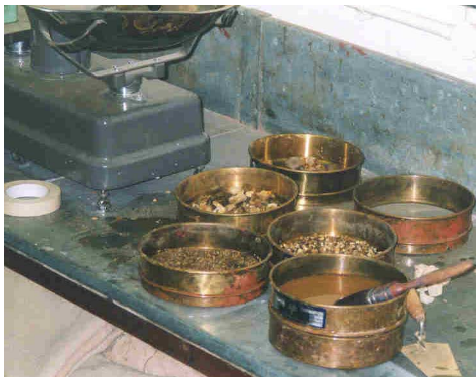
Figure 3.2 – Wet sieving is the standard soil classification method
