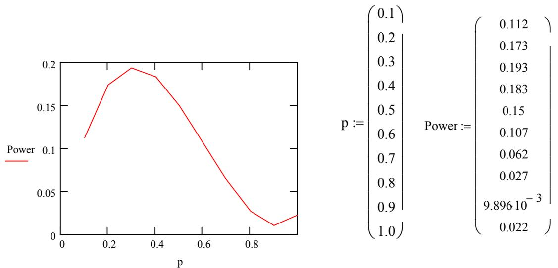
ii) Values of p from 0.20-0.39 were plotted against Power Output values (kW) with the maximum occurring at 0.3 confirming the proof work in the Technical Background chapter
