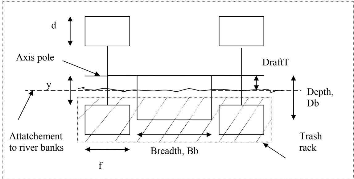
Fig. 43 Cross section showing barge with two waterwheels attached at either side
