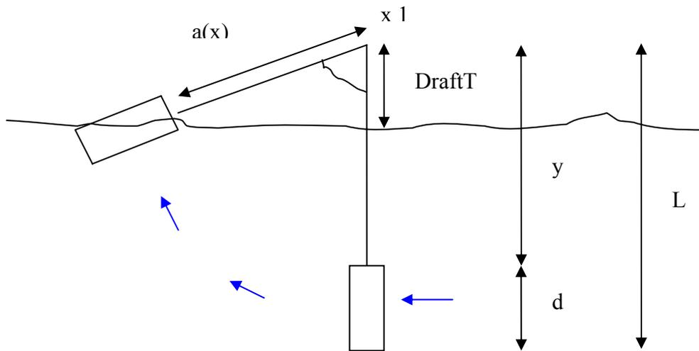
Fig. 30 Diagram showing the passage of one blade through the water
