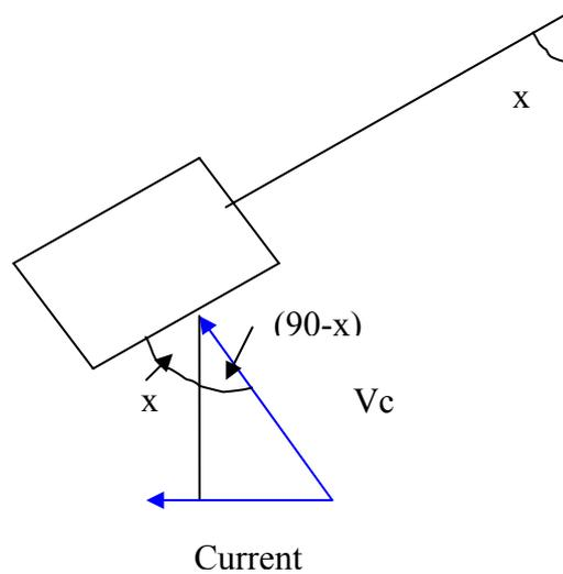
Fig... Diagram showing the current component in the blade's direction,  $V_c$
