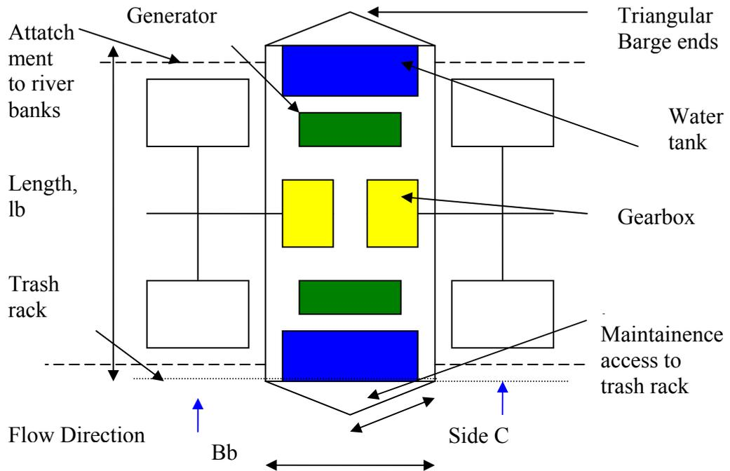
Fig. 44 Plan of barge showing approximate layout of generator, gearbox and watertanks
