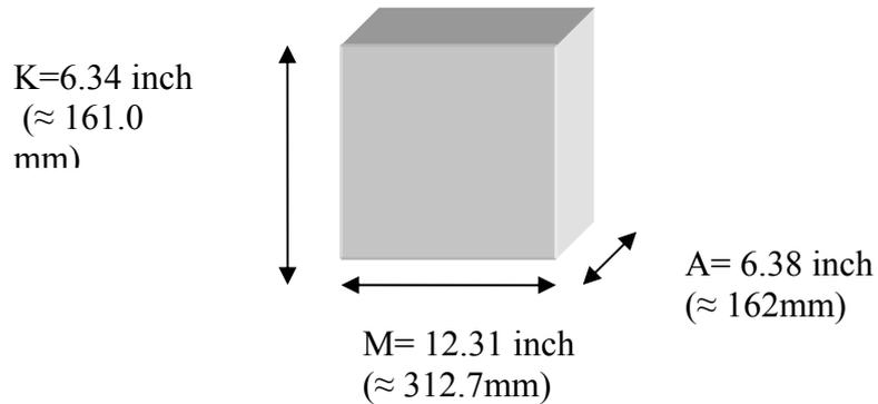
Fig. 46 Overall dimensions of gearbox from (51)
