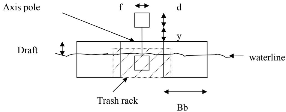
Fig. 50 Cross section of catamaran in direction of flow
