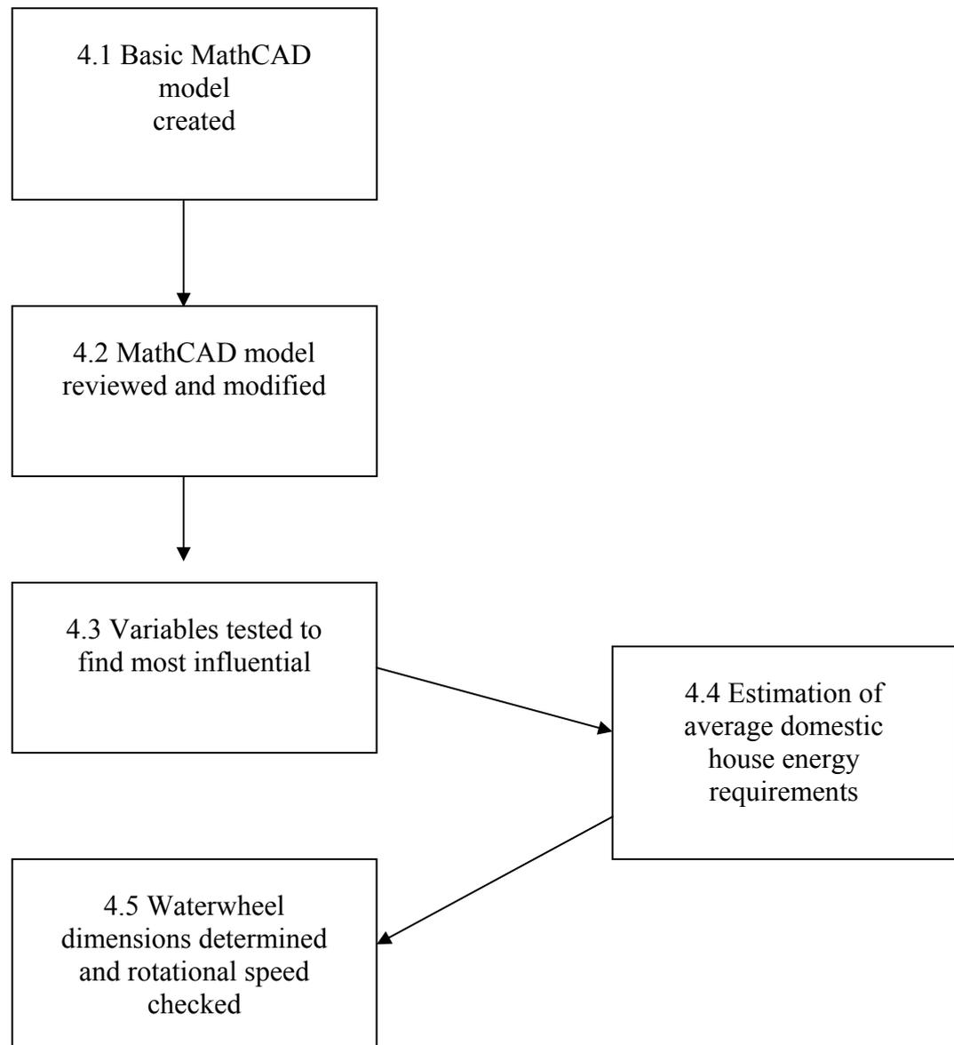
Fig. 32 Design process for waterwheel
