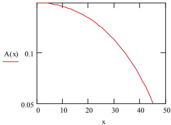
As the Force output is based on the Area this graph will give a low output as the area is decreasing with x. A more optimum design would have a constant area for as long as possible and then a quick drop in submerged area
