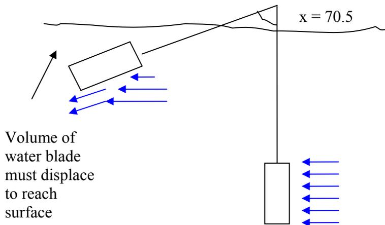
Fig. 38 Diagram showing blades at 0 degrees and 70.5 degrees.
