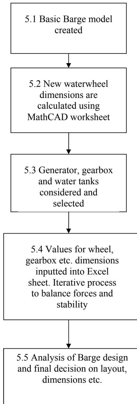
Fig. 42 Design process for barge
