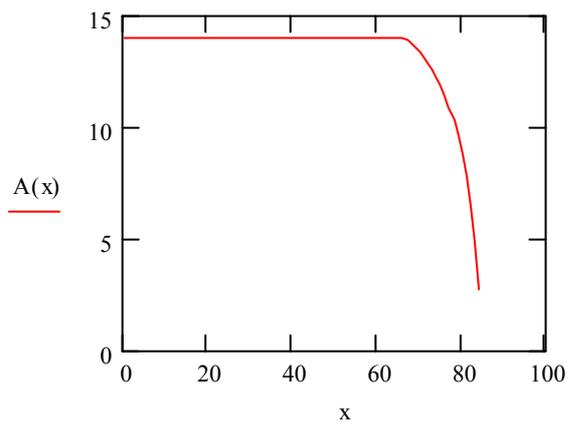
The inclusion of a DraftT term allows the Area to be accurately calculated. The graph above shows the blade area being constant, as it moves through the water and then suddenly dropping as it leaves the water
