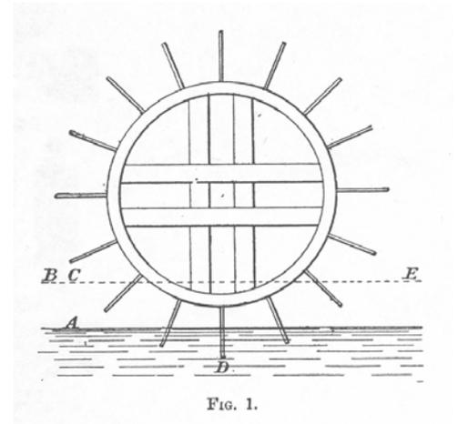
As this is less than the potential energy the stream wheel is often regarded as being inefficient, however interest has resurged in them as “*their application does not constitute a major change of river*” (25). No civil works are required, the wheel can be moored on a barge or fixed to the side, and the relatively simple dimensions and layout mean that it can be constructed and repaired locally, lending itself more to the developing world than the Zuppinger wheel.
