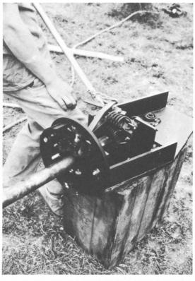
Figure 4.35. The brake reset lever.
