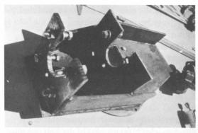
Figure 4.16. The Sailwing hub assembly and crank-shaft mount.
