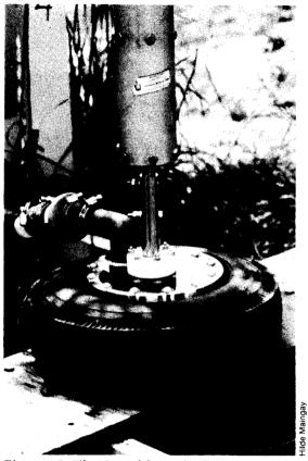
Figure 4.5. The New Alchemy diaphragm tire pump.
