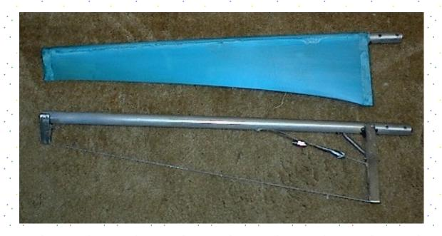
The above blade was built in under 20 minutes using the "tube and wire" method. That's from cutting materials to the blue assembly. It will still need paint but all 3 blades can be built in about an hour. The blade will follow a twist from 2 degrees at the tip down to 23 degrees at the tip. Its set to run at a TSR of around 6 and is
