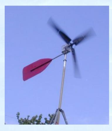
The result is a a bit more speed in the gusts. As I write this we're having winds with gusts up over 20 mph, and I'm seeing an easy 1 to 1 1/2 amps going into the batteries on the average, more in the strongest peaks. This is certainly not bad for a little NEMA 34 stepper motor. I have a feeling that it will do better in some real wind, at least as long as it holds together.
