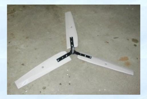
I found a scrap of heavy guage steel about 1 1/2" wide, and cut it into three equal strips about 7 inches long. These I sandwiched between two very large washers. A bolt and nut squished the washers together, capturing the steel strips. Once they were perfectly aligned, I welded them all together, forming a solid three-blade hub.
