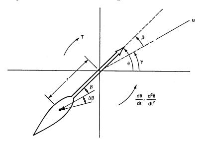
Figure 13: Wind vane angles
