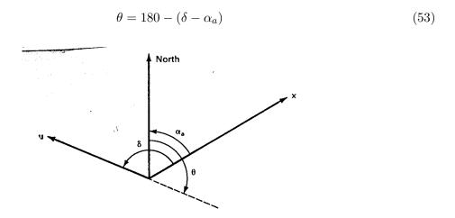
Figure 20: Geometry for computing wind direction.
