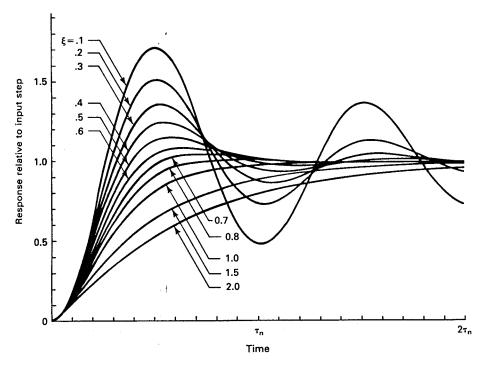
Figure 15: Second-order system response to a step input
