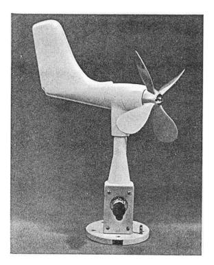
Figure 2: Propeller-type wind-speed sensor. (Courtesy of Weathertronics, a Division of Qualimetrics, Inc., P.O. Box 41039, Sacramento, CA 95841.)
