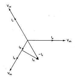
Figure 19: Phasor diagram for circuit in Fig. 18 at balanced operation at unity power factor.
