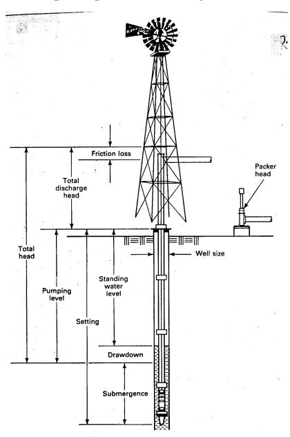
Figure 1: Aermotor illustration of key water pumping terms.
