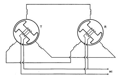
Figure 11: Synchro wind direction transmitter and receiver.
