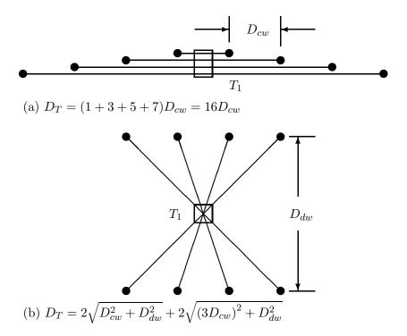
Figure 3: Trench lengths for low voltage wiring for 8 turbines in  $1 \times 8$  and  $2 \times 4$  configurations.
