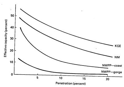
Figure 25: Wind power plant effective capacity versus penetration.
