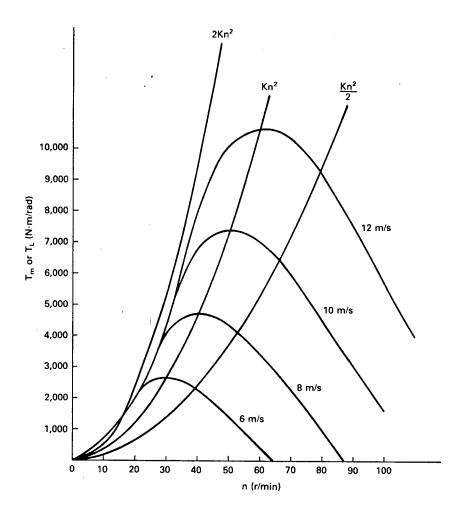
Figure 29: Three loads attached to Sandia 17-m turbine.
