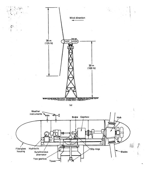
Figure 1: NSF–NASA MOD-0 wind power system: (a) general view; (b) superstructure and equipment. Rated power output, 100 kW; rated wind speed, 8 m/s (18 mi/h). (Courtesy of DOE.)
