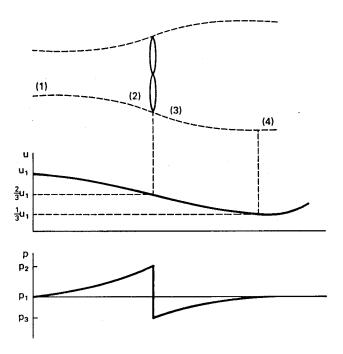
Figure 2: Circular tube of air flowing through ideal wind turbine.
