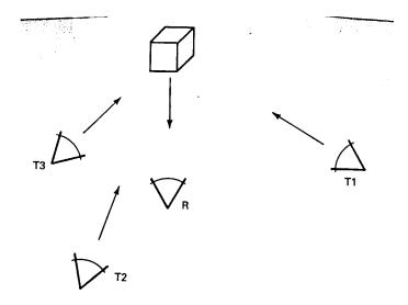
Figure 8: Doppler acoustic radar configuration.
