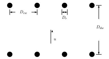
Figure 1: Dimensions of Turbines in a Windfarm
