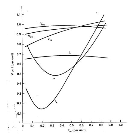
Figure 21: Variation of line-to-line voltages and line currents of 40-hp induction generator connected in circuit of Fig. 18.  $R_L = 3.72$  pu, C = 1.09 pu.
