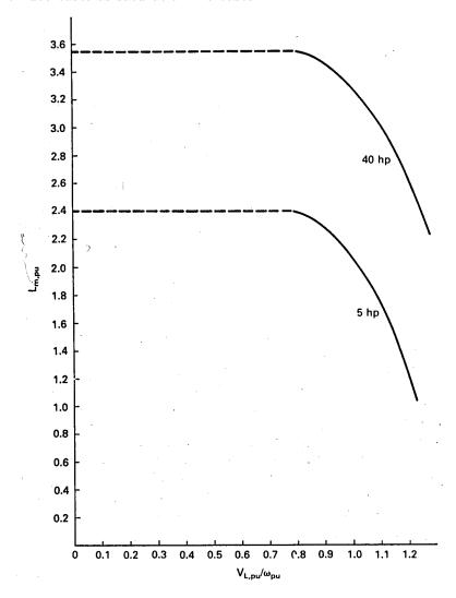
Figure 13: Per unit magnetizing inductance as a function of load voltage.
