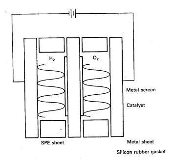
Figure 18: Solid polymer electrolyte electrolysis cell.
