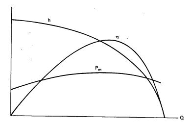
Figure 5: Pump characteristics of head, efficiency, and input power as a function of capacity at constant speed.
