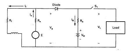
Figure 2: DC shunt generator in a battery-charging circuit.
