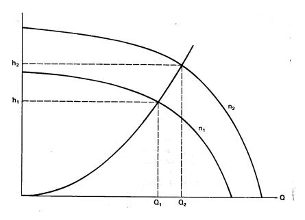
Figure 6: Head versus capacity curves for two different speeds.
