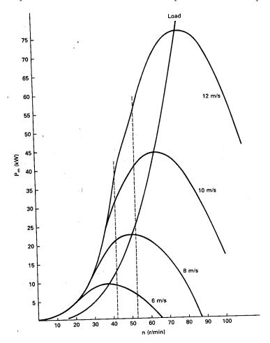
Figure 26: Shaft power output of Sandia 17-m Darrieus in variable-speed operation.
