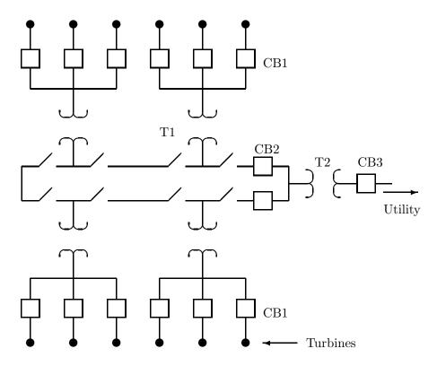
Figure 2: One Line Diagram of Windfarm Electrical Network
