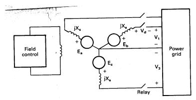
Figure 13: AC generator being synchronized with the power grid.
