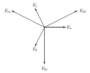
Figure 7: Balanced three-phase voltages for circuit in Fig. 5.6.
