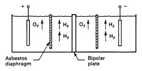
Figure 14: Two electrolysis cells in series.
