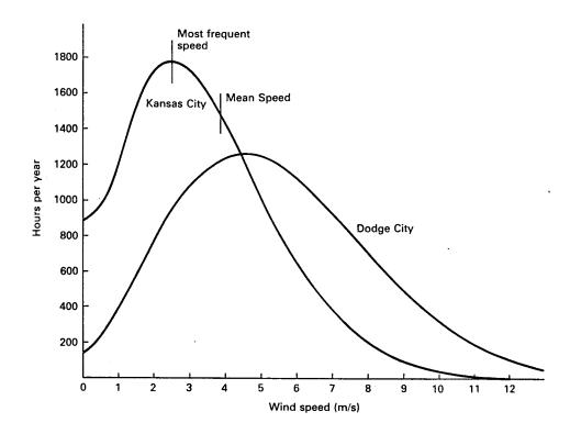
Figure 7: Speed-frequency curves, 1970
