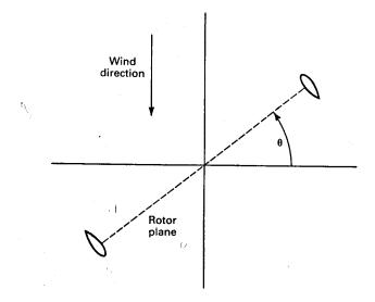
Figure 21: Definition of rotor angle for Sandia 17-m Darrieus.
