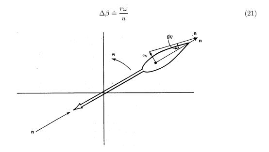
Figure 14: Effective direction of wind due to vane rotation.
