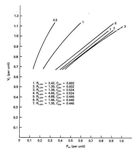
Figure 14: Variation of output voltage with input shaft power for various resistive and capacitive loads for a 40-hp self-excited induction generator.
