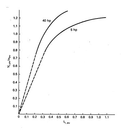
Figure 12: No-load magnetization curves for two induction generators.
