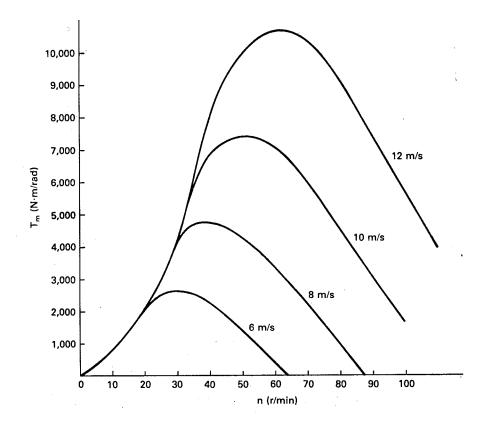
Figure 27: Shaft torque output of Sandia 17-m Darrieus in variable-speed operation.
