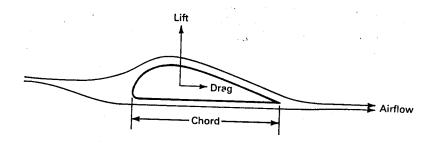
Figure 3: Lift and drag on a stationary airfoil.
