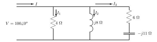
Figure 5: Parallel *RLC* circuit.
