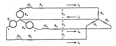
Figure 5: Permanent-magnet generator connected to a resistive load.
