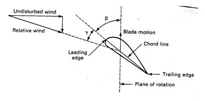
Figure 6: Definition of pitch angle  $\beta$  and angle of attack  $\gamma$ .
