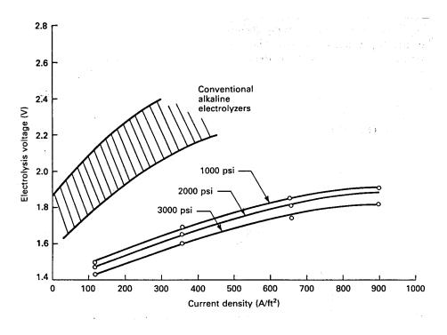
Figure 16: Plot showing the effect of pressure on electrolysis cell characteristics at 400°F.
