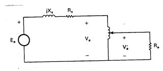
Figure 6: Load adjustment with a variable autotransformer.
