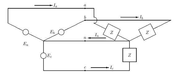
Figure 8: Balanced three-phase wye-connected source and load.
