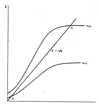
Figure 3: Magnetization curve of dc generator.
