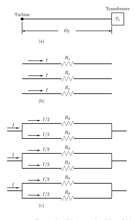
Figure 5: Loss Calculation in Low Voltage Cable
