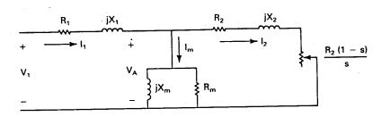
Figure 17: Equivalent circuit for one phase of a three-phase induction motor
