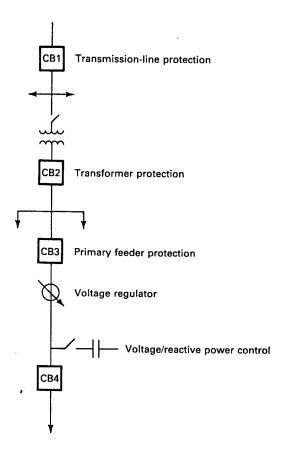
Figure 27: Distribution substation protection.
