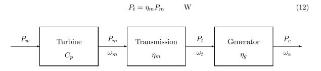
Figure 12: Wind electric system
