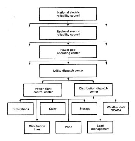
Figure 28: Monitoring and control hierarchy.
