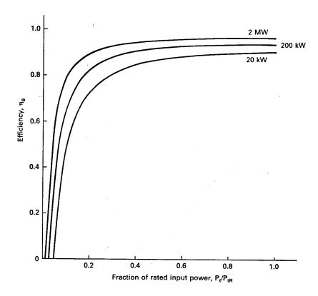
Figure 14: Generator efficiency for three generator sizes.
