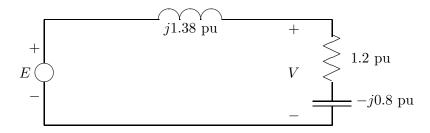
Figure 14: Per phase diagram for example problem.
