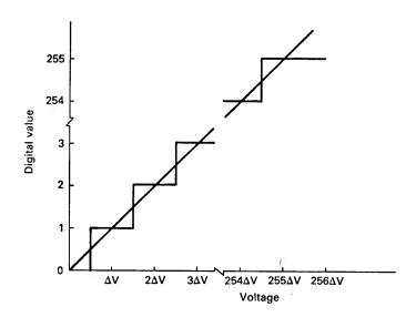
Figure 5: Digital representation of analog voltages.
