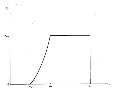
Figure 16: Model wind turbine output versus wind speed.
