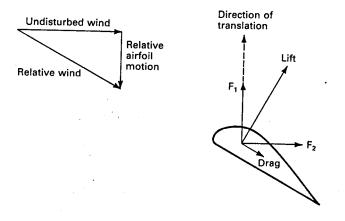
Figure 4: Lift and drag on a translating airfoil.
