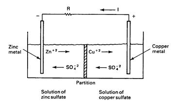
Figure 9: Zinc-copper voltaic cell.
