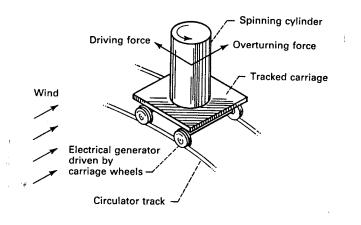
Figure 10: Madaras concept for generating electricity.
