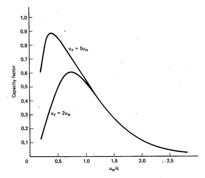
Figure 18: Wind turbine capacity factor as a function of rated speed.  $u_c = 0.5u_R$  and k = 2.
