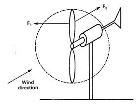
Figure 5: Aerodynamic forces on a turbine blade.
