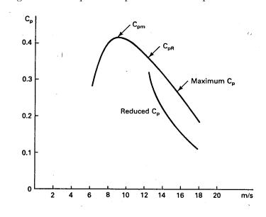
Figure 8: Coefficient of performance versus wind speed for MOD-2.
