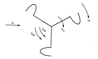
Figure 6: Torques or moments existing on a cup-type anemometer.
