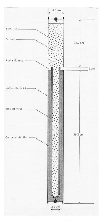
Figure 13: Beta battery cell. (©1979 IEEE)
