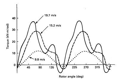
Figure 20: Aerodynamic torque variation for Sandia 17-m Darrieus at 50.6 r/min.
