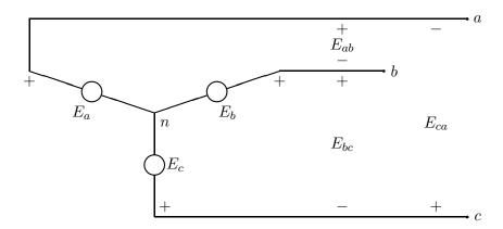
Figure 6: Balanced three-phase source.
