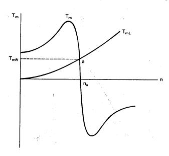
Figure 18: Variation of shaft torque with speed for a three-phase induction machine.
