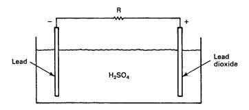
Figure 10: Lead-acid voltaic cell.
