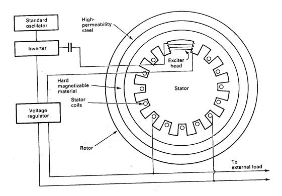
Figure 24: Basic diagram of Roesel generator.
