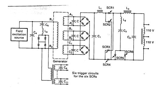
Figure 23: Simplified schematic of field-modulated generator.
