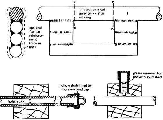
Fig. 36 Grease lubrication systems for wooden bearings
