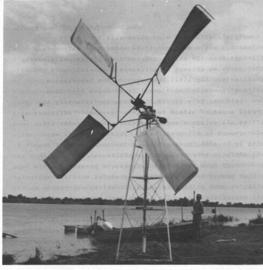
Fig 16. Experimental 18ft diameter four-sail wind-mill with feathering blades operating downwind of the tower.
