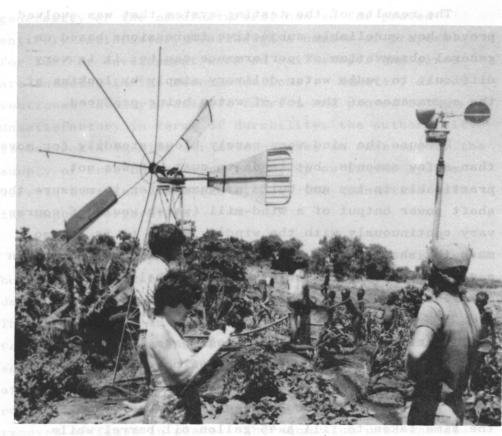
Fig 25. Windmill testing by filling a 45 gallon barrel (metal blades being evaluated).
