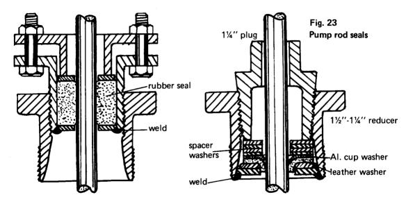
Fig 23. Alternative pump rod seals.
