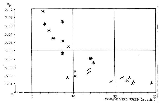
This graph suggests that the  $C_p$  (coefficient of performance) is influenced more by the wind speed than by the number of sails fitted - provided sufficient sails are fitted to give reliable operation.
